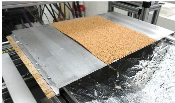
Figure 69 - The transport plate with the PEEK brush at the side walls and an insulating plate of cork in the depression for drying experiments is shown.
