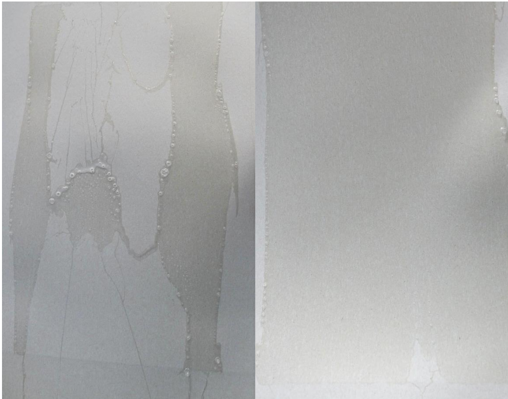
Figure 124 - RS2 Std. coated substrate. \dot{V}_l = 1.08 \text{ l/min} , v_{sub} = 2.6 \text{ m/s} , v_{imp} = 1.07 (left) and 1.24 \text{ m/s} (right).
