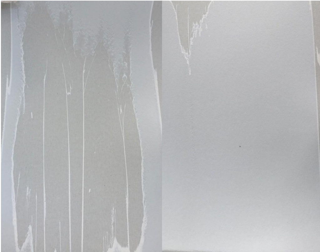
Figure 126 - RS3 Std. coated substrate. \dot{V}_l = 0.86 \text{ l/min} , v_{sub} = 4.59 \text{ m/s} , v_{imp} = 1.18 \text{ m/s} (left) and \dot{V}_l = 0.81 \text{ l/min} , v_{sub} = 4.33 \text{ m/s} , v_{imp} = 1.33 \text{ m/s} (right).
