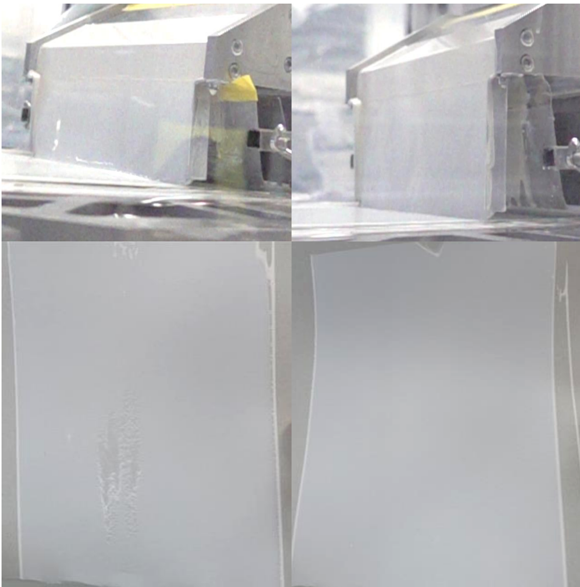
Figure 84 - RS3 Std. impingement velocity effect. Left column: \dot{V}_l = 0.93 \text{ l/min} , v_{imp} = 1.18 \text{ m/s} , v_{sub} = 3.7 \text{ m/s} ; Right column: \dot{V}_l = 0.93 \text{ l/min} , v_{imp} = 1.33 \text{ m/s} , v_{sub} = 3.8 \text{ m/s} .
