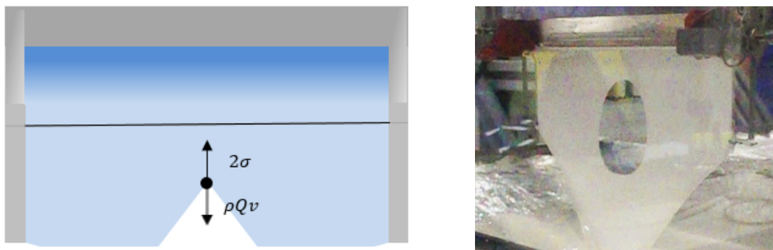
Figure 9 - Disintegrating curtain. Force balance that shows: Inertia of falling liquid sheet must balance surface tension of both free surfaces (left). Growing hole in a curtain (right).
