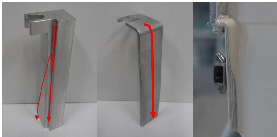
Figure 53 - Edge guide designs with original edge guide geometry (left), proposed edge guide geometry (mid) and proposed edge guide geometry during the process (right). The arrows indicate liquid flow.
