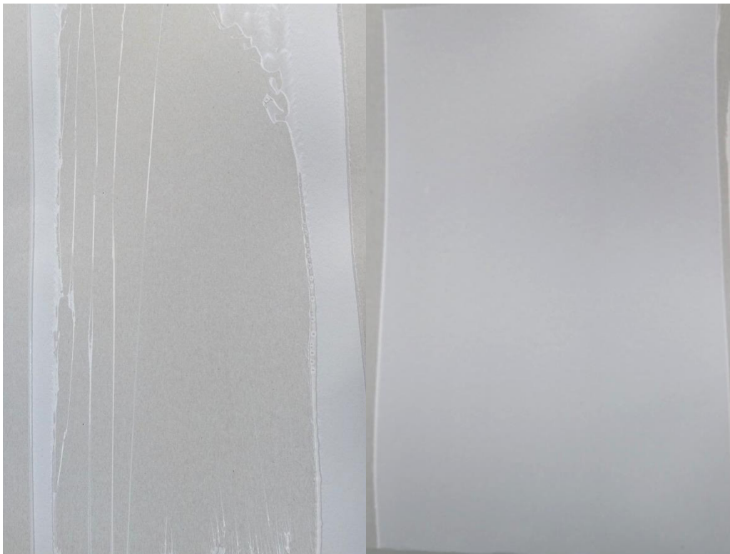
Figure 127 - RS3 Std. coated substrate. \dot{V}_l = 0.91 \text{ l/min} , v_{sub} = 3.90 \text{ m/s} , v_{imp} = 1.16 \text{ m/s} (left) and \dot{V}_l = 0.91 \text{ l/min} , v_{sub} = 4.20 \text{ m/s} , v_{imp} = 1.33 \text{ m/s} (right).
