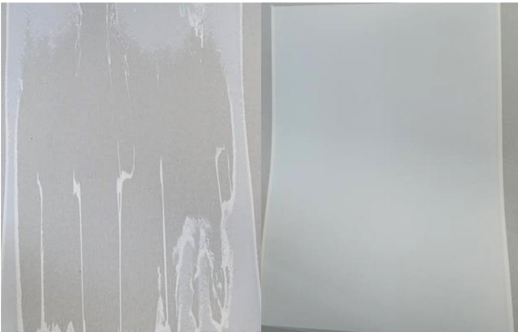
Figure 82 - RS3 Std. Coating results. Left: \dot{V}_l = 0.85 \text{ l/min} , v_{imp} = 1.18 \text{ m/s} , v_{sub} = 5 \text{ m/s} ; right: \dot{V}_l = 1.10 \text{ l/min} , v_{imp} = 1.18 \text{ m/s} , v_{sub} = 1.7 \text{ m/s} .
