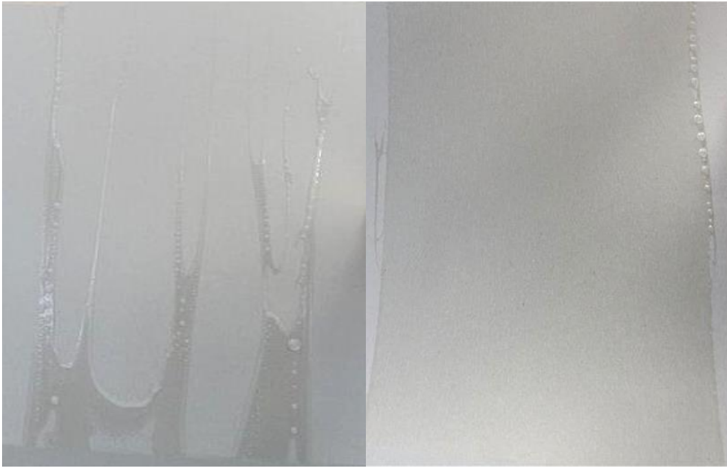
Figure 81 - RS2 Std. Coating result. Left: \dot{V}_l = 0.70 \text{ l/min} , v_{imp} = 1.07 \text{ m/s} , v_{sub} = 1.8 \text{ m/s} ; right: \dot{V}_l = 2.50 \text{ l/min} , v_{imp} = 1.08 \text{ m/s} , v_{sub} = 5 \text{ m/s} .
