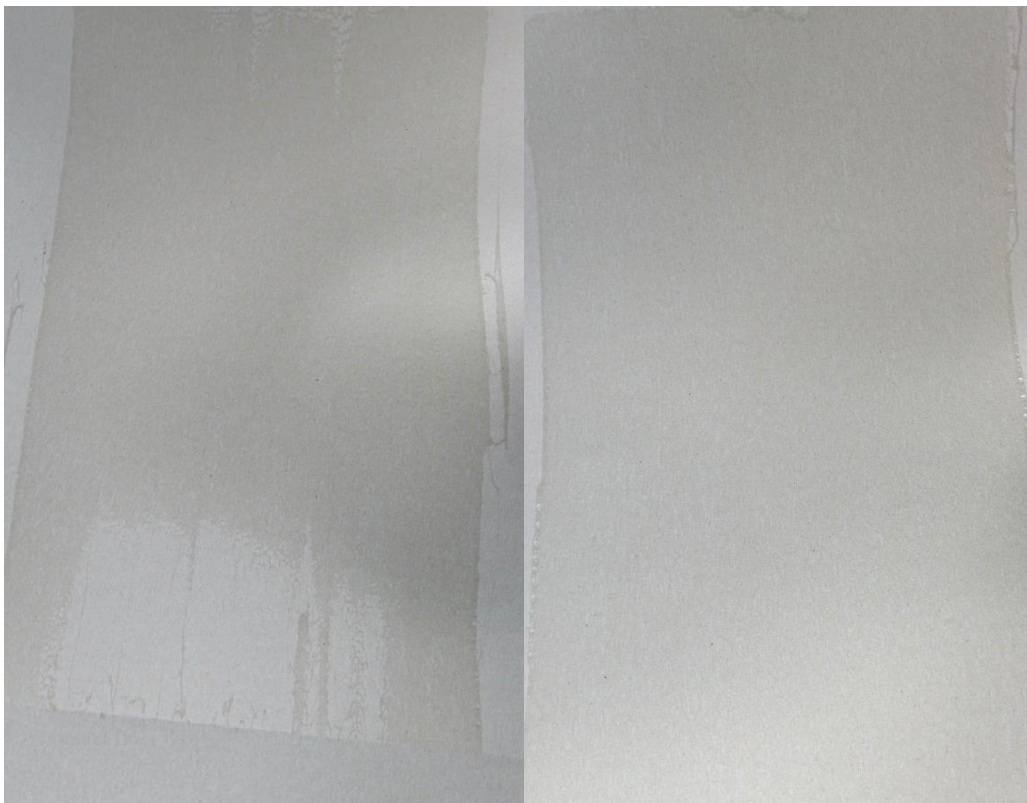
Figure 125 - RS2 coated substrate. \dot{V}_l = 1.55 \text{ l/min} , v_{sub} = 5 \text{ m/s} , v_{imp} = 1.07 (left) and 1.24 \text{ m/s} (right).
