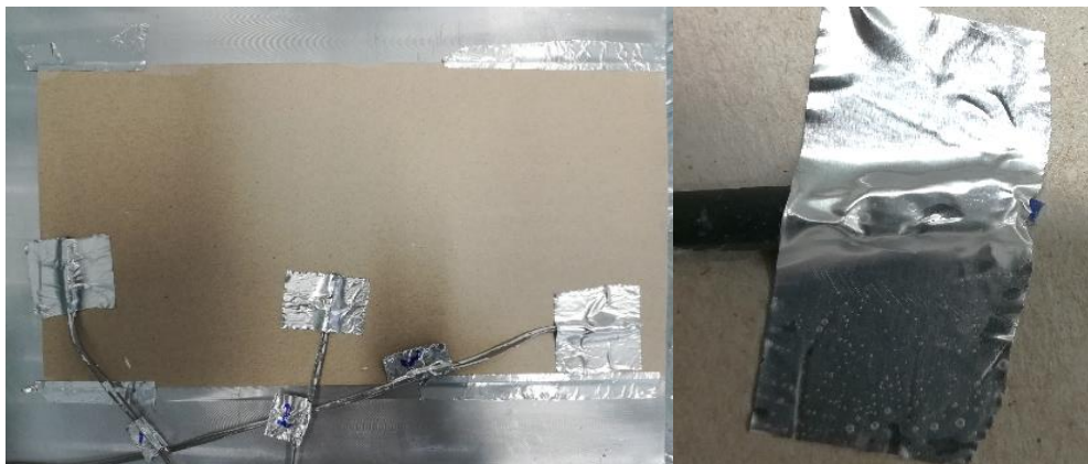
Figure 78 - Substrate with temperature sensors of the MTME at specified positions (left) and correctly fixed sensor with the tip not fully covered by the tape (right).
