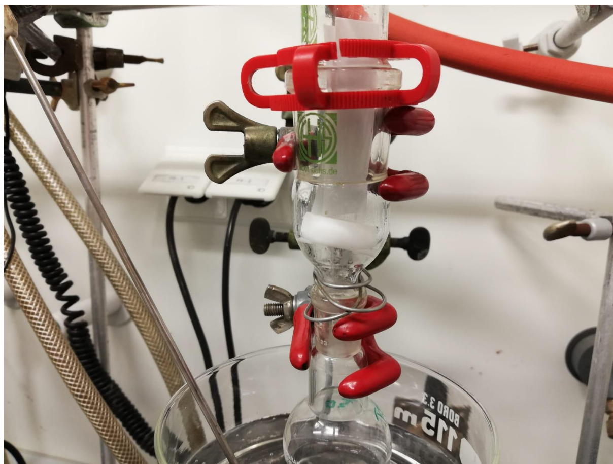
Figure 10: Enlarged picture of the reaction chamber consisting of a reduction combined with an olive. A Teflon disc with little holes is used to keep the paper sheets in the right position.
