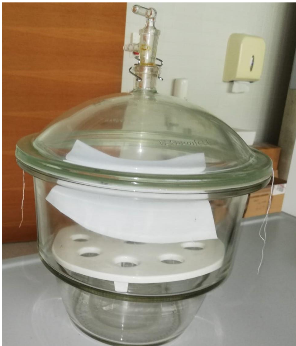
Figure 11: Scaled up setup to hydrophobize larger paper sheets in a desiccator. The paper sheet was hung up via a yarn and the sizing agent was placed in a glass bowl under the intermediate base.
