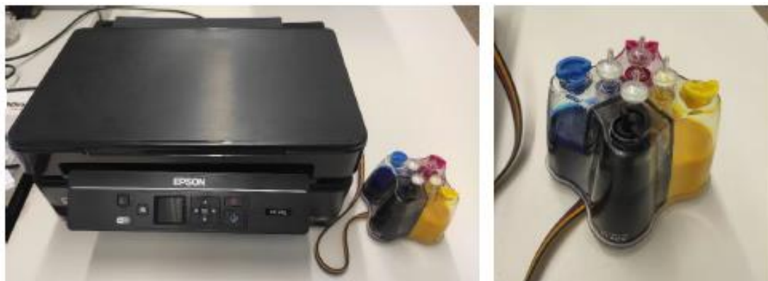
Figure 14: Epson printer and ink tank system for the printing tests. Picture taken from [74].
