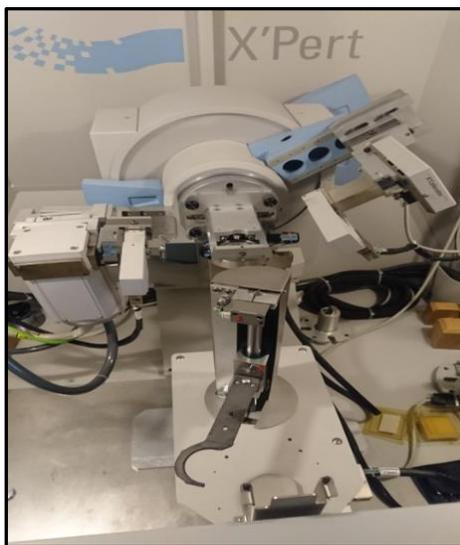
Figure 12: Sample changer and measurement device inside the Panalytical X'Pert Pro
