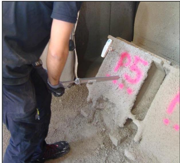
Figure 19: Needle Penetration Test carried out in Wopfung
