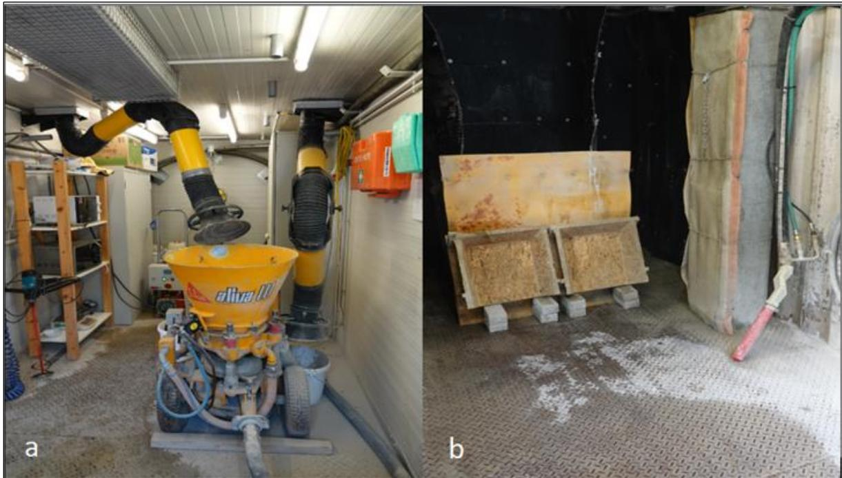
Figure 18: a: Mixing device in one of the containers in Wopfing. b: Wooden boxes, where the shotcrete was sprayed and red nozzle of the spraying device.
