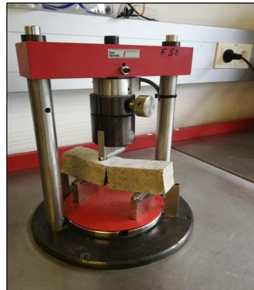
Figure 9: ToniPRAX flexural strength testing machine at TU Graz Inffeldgasse
