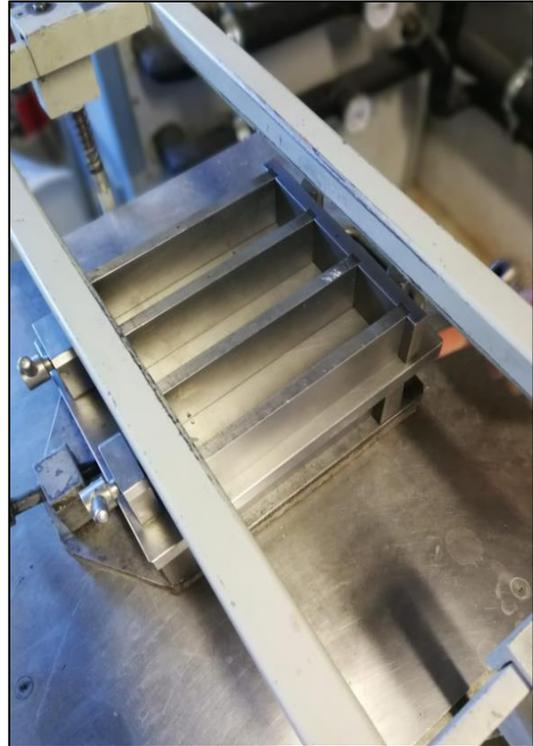
*Figure 10: Prism-steel-case placed on the shaker before the mortar was poured in.*
