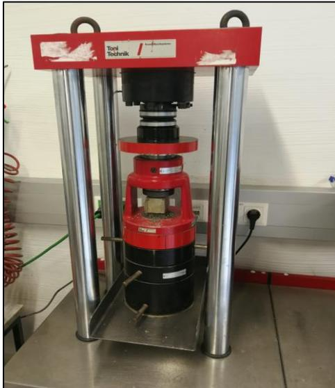
Figure 8: ToniPRAX compressive strength testing machine at TU Graz Inffeldgasse
