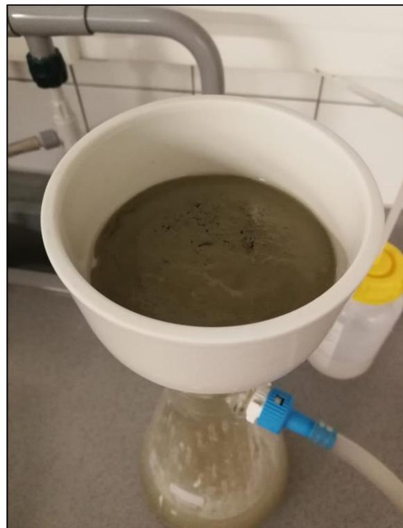
Figure 17: CEM I reference mix on the cellulose filter after the addition of isopropanol. Glass container underneath is under vacuum.
