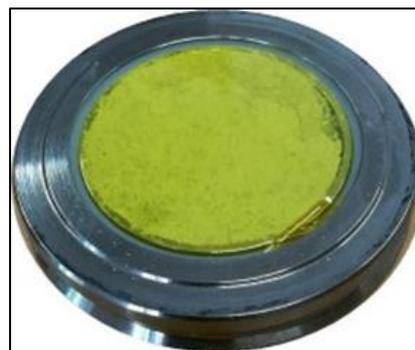
Figure 14: Kapton film on a sample used for a 24h In-situ measurement
