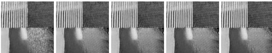
Figure 3.12: Results for different numbers of iterations for the mix image with p = 40\% and \lambda_{\text{TV}} = 1.8 . From left to right, number of iterations is: 100, 500, 1000, 2500, 5000.
