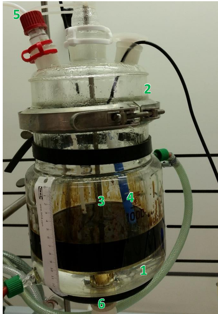
Figure 10. Set up of the lab-scale precipitation reactor. The reactor (here shown charged with BL) consists of a glass vessel with heating jacket (1), glass lid (2), propeller (3), pH electrode and temperature sensor (4), CO 2 inlet pipe (5), bottom outlet (6).
