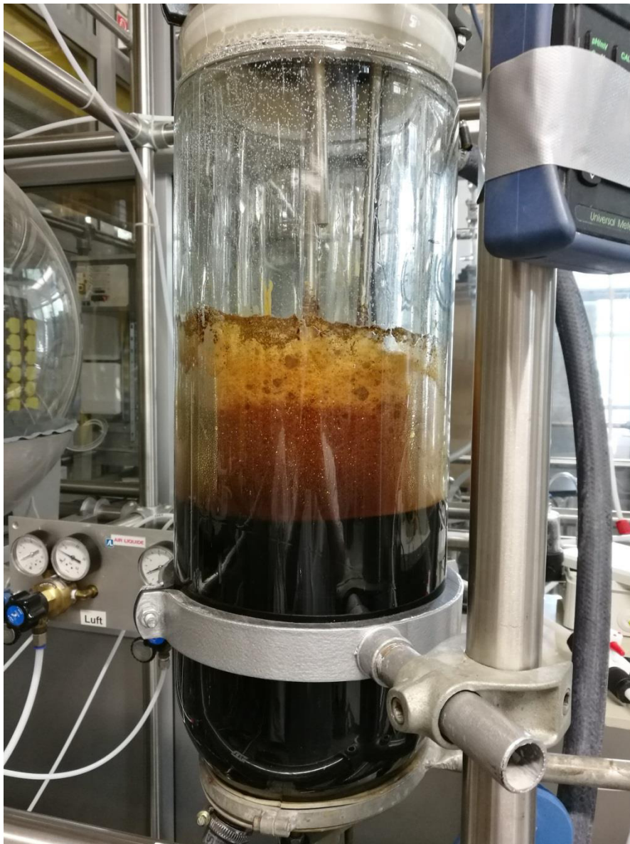
Figure 11. Pilot-scale precipitation reactor filled with BL. Introduction of dilute CO 2 gas led to the formation of foam above the liquid surface.
