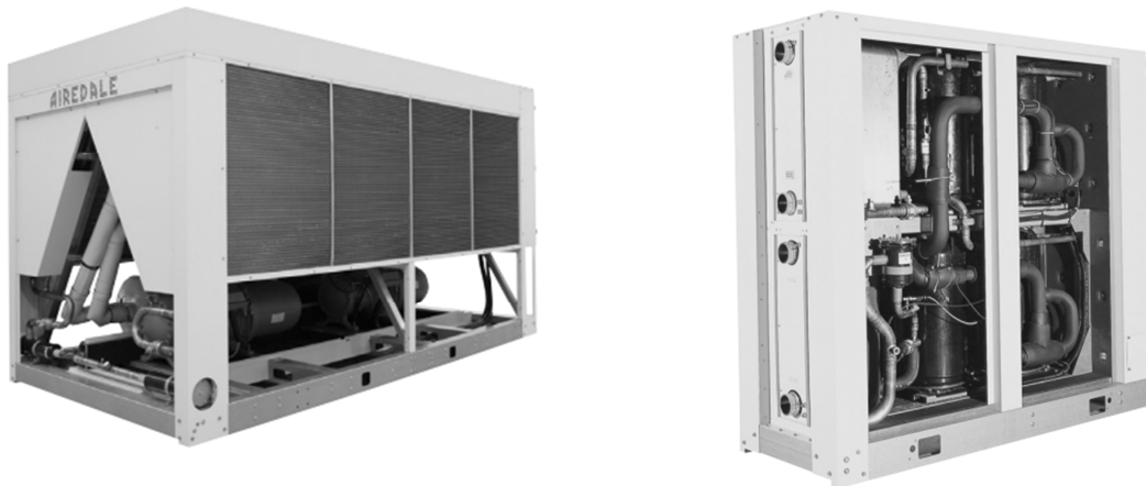
Figure 2-24: Air-cooled 600 kW chiller (left) and water-cooled 250 kW chiller (right) 115
