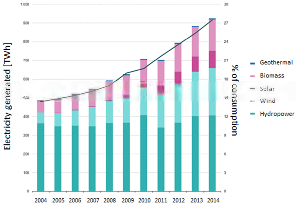
Figure 3-2: Development of the electric power generated by renewable energy sources 240
