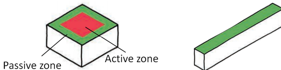
Figure 3-4: Deep plan (left) versus Shallow plan (right) 262
