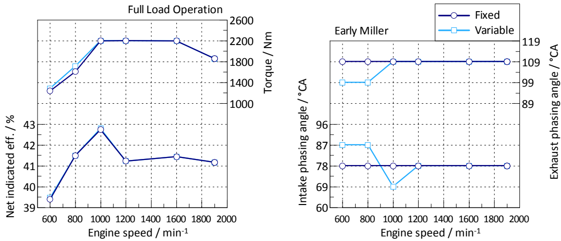
Figure 5.34: Right: Derived operating strategy of cam phasing at full load operation in combination with the early Miller cam profile. Left: The effect of cam phasing on the engine torque and the net indicated efficiency.
