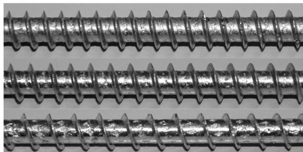
**Figure 3.49:** Photographs of self-tapping screws' threaded parts produced by manufacturers A, B and C
