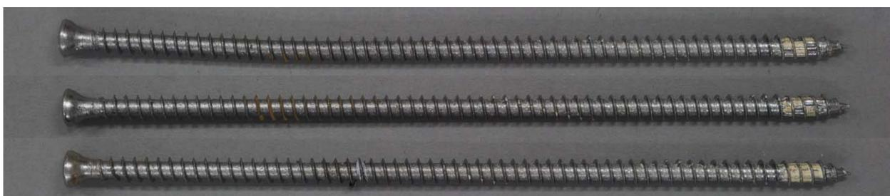
**Figure B.10:** *Macrophotos of A\_s\_IV\_08\_240 (zinc-nickel) applied in Norway spruce; test campaign I; according to Hauptmann (2016)*
