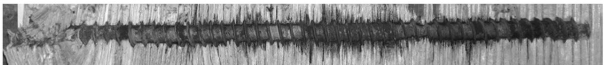
**Figure 3.82:** Opened timber specimen (oak) with *A\_s\_I\_08\_240* (yellow chromated) failed in the frame of test campaign I
