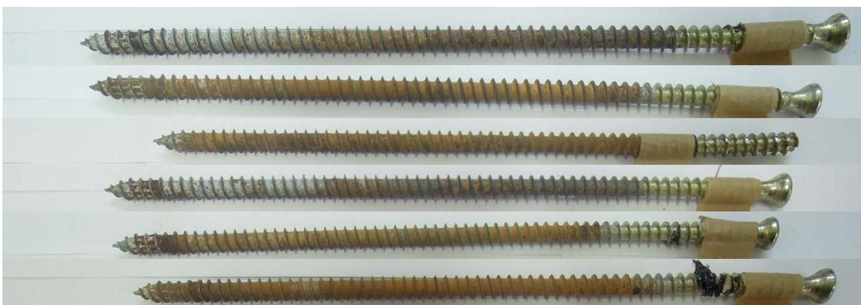
**Figure B.11:** *Macrophotos of A\_s\_II\_08\_240 (yellow chromated) applied in oak; test campaign II*
