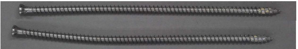
**Figure B.6:** *Macrophotos of A\_s\_I\_08\_240 (zinc-nickel) applied in Norway spruce; test campaign I; according to Hauptmann (2016)*
