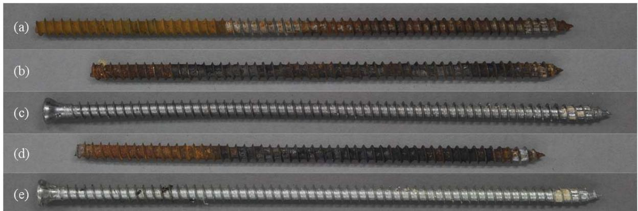
**Figure 3.78:** *Macrophotos of test campaign I: (a) yellow chromated in oak; (b) zinc-nickel in oak; (c) zinc-nickel in Norway spruce; (d) blue chromated in oak; (e) blue chromated in Norway spruce; according to Hauptmann (2016)*
