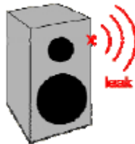
Figure 17: Leakage in the enclosure (Klippel 2010)
