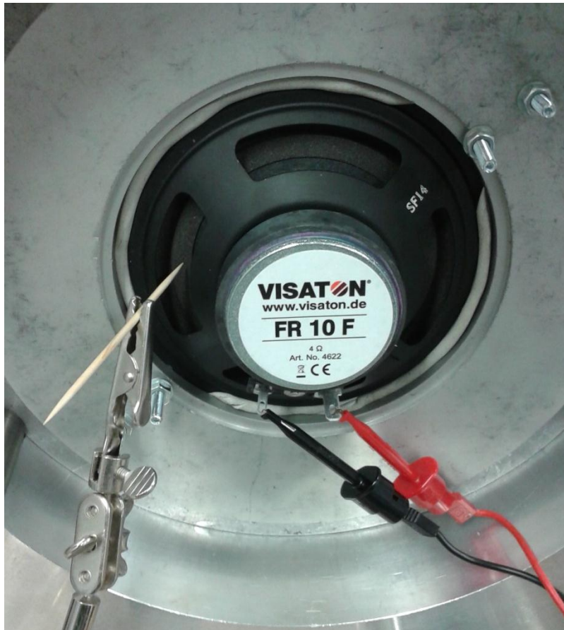
Figure 87: A toothpick next to the membrane at the backside to generate a hitting membrane
