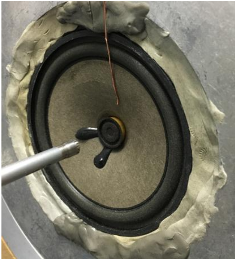
Figure 110: Loudspeaker with a fixed wire at the front to simulate a buzzing wire loop
