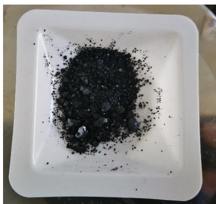
Figure 18: The dried amorphous \text{MnO}_2 precursor.
