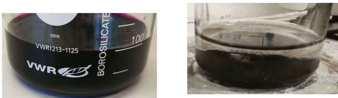
Figure 19: \text{MnO}_2 precursor mixed with \text{CoCl}_2 \cdot 6 \text{H}_2\text{O} (left), the resulting product after the reduction with \text{NaBH}_4 (right).
