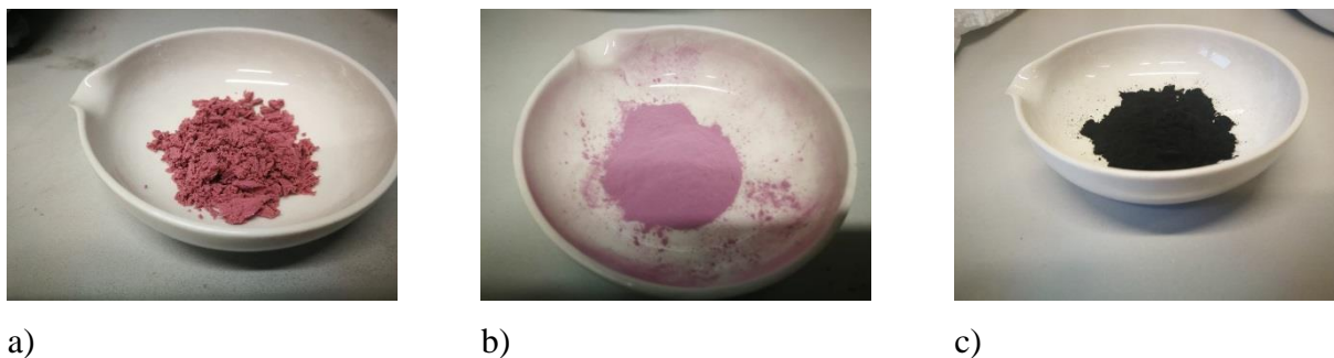
Figure 21: The Co_{0.33}Mn_{0.67}CO_3 precipitate before (a) and (b) after drying at 60^\circ C and (c) after annealing at 400^\circ C to obtain CoMn_2O_4 .
