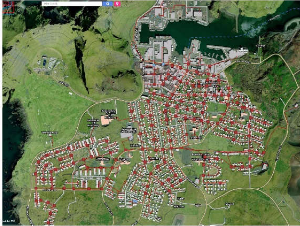
Figure 17, Geothermal distribution network in the small town of Heimaey in Iceland, district heating based on GE found in the preceding local lava eruption, clever method of attaining benefits from a disaster. Iceland is one of the most potent countries with GE, source: www.verkis.is , presentation by T. Johansson, Cornell University, November 2016, courtesy of the presenter
