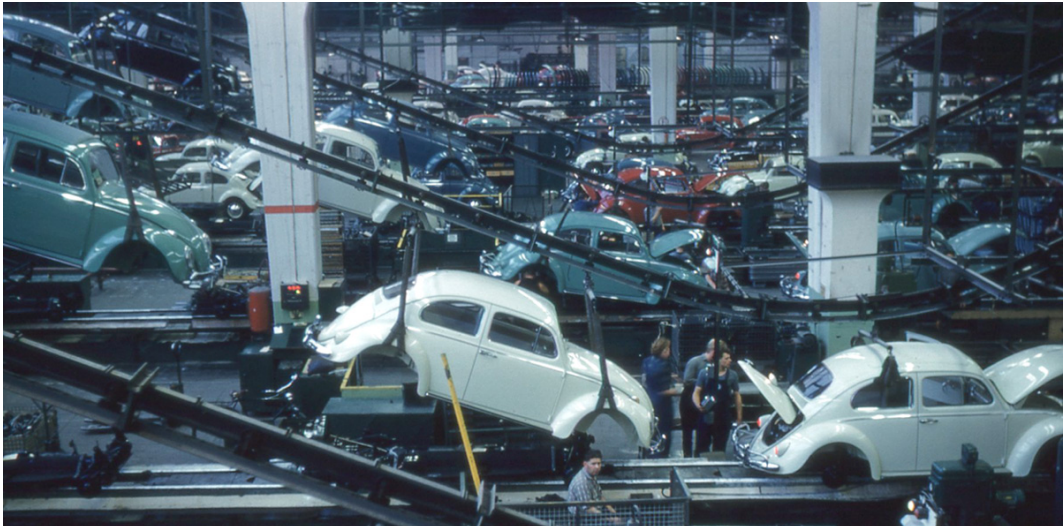
Figure 1.1: Fixed assembly line of Volkswagen Beetle. Source: https://w.wiki/PXi
