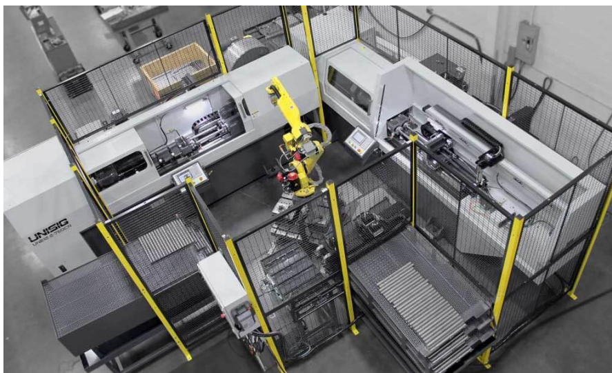
Figure 2 Part of a Flexible Machining System (Unisig 2018)
