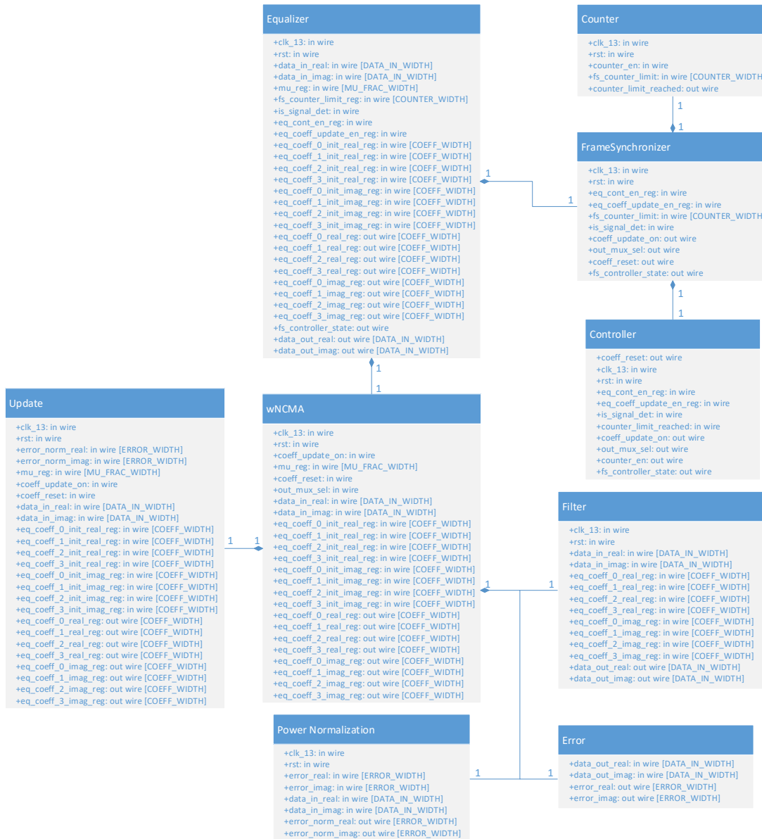
Figure 3.3: UML Class Diagram of the wNCMA equalizer. Each class represents a Verilog module.
