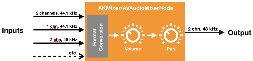
Figure 7.2: Visualization of AKMixer 's/ AVAudioMixerNode 's functionality
