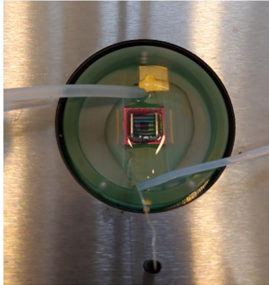
Figure 3.3: Chip during recording, on the left side top the inflow, right bottom drain, in the middle bottom the reference electrode within in the solution. The slice is fixed with a platinum wire.
