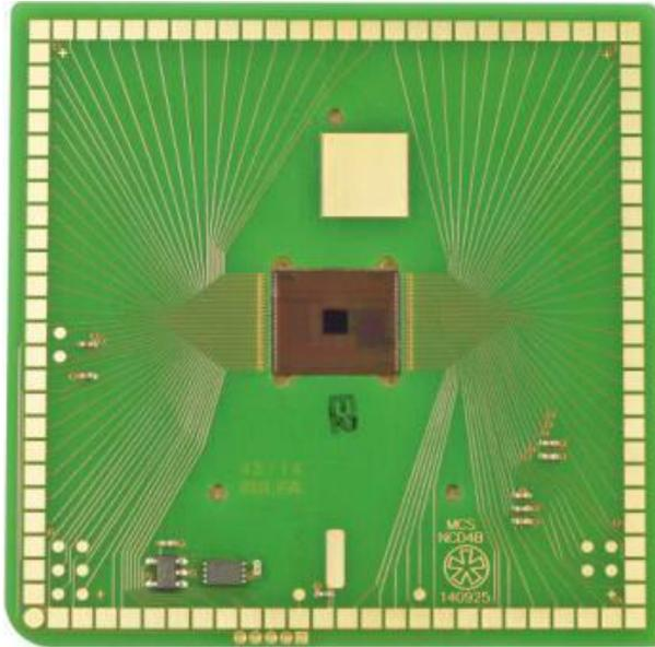
Figure 1.10: CMOS chip with 4225 recording and 1024 stimulation electrodes. [29]
