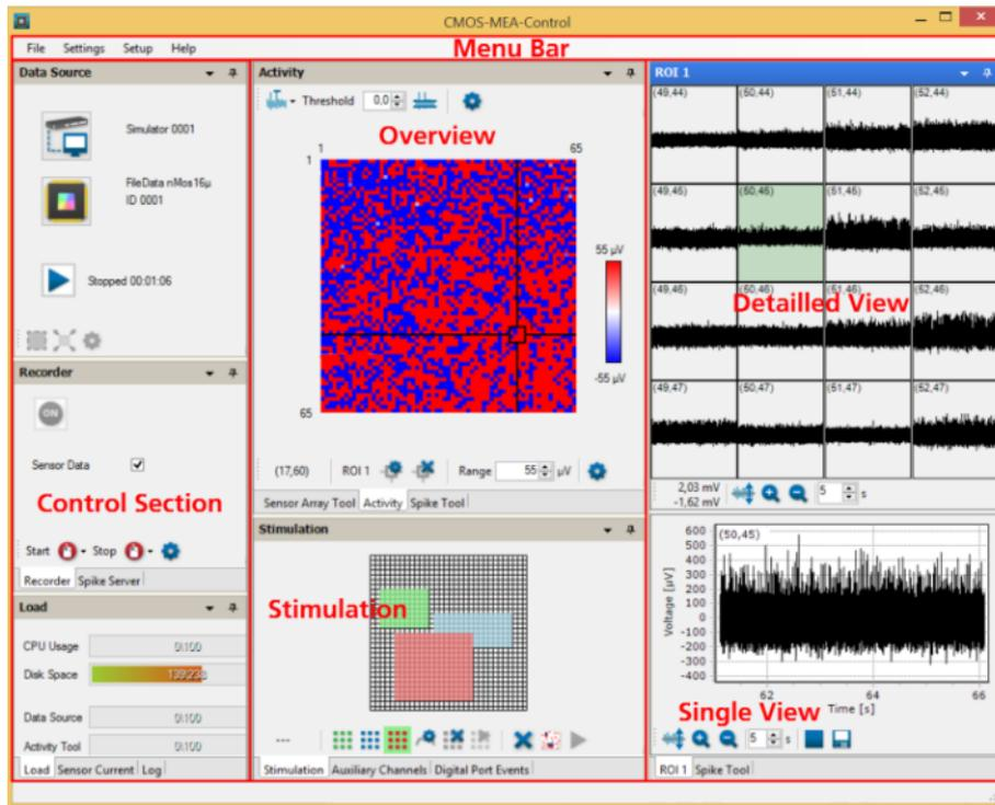
Figure 3.4: CMOS-MEA control software overview. Control section on the left side shows general information, the overview in the middle displays the chip array and the stimulation to trigger an impulse. The right side detailed view visualizes a small number of electrodes and the single view displays only one electrode. [16]
