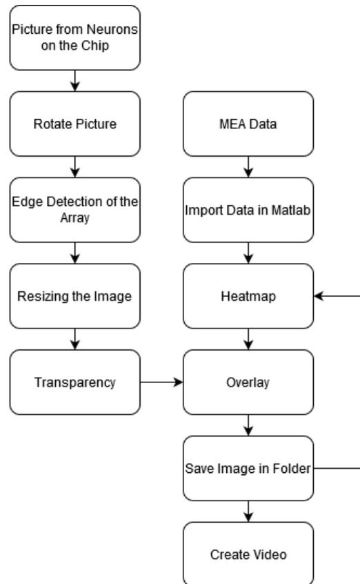
Figure 3.9: Flowchart describing all steps of the code for dissociated neurons in Matlab, from import to the final part the video.
