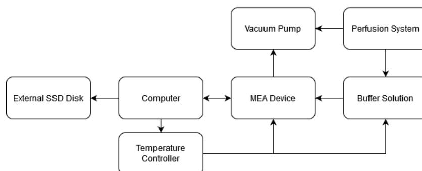
Figure 3.1: Measurement setup arrows display how the devices interact with each other
