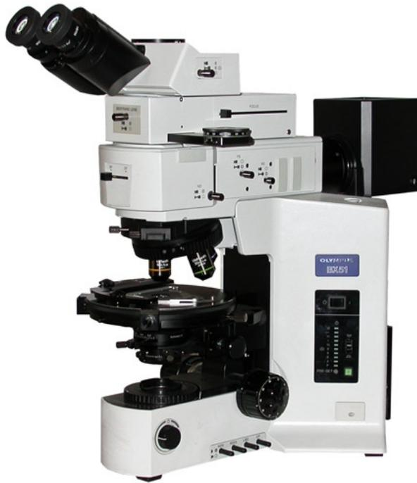
Figure 1.5: Olympus reflected-light microscope. [24]
