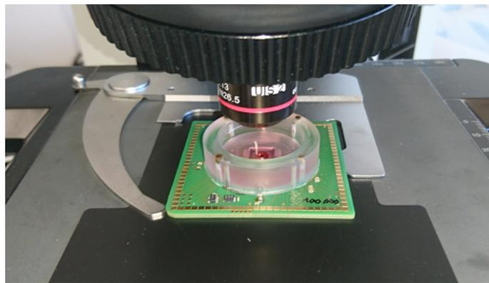
Figure 3.7: Recording images from hippocampal slices or neurons by microscope from Olympus, mounting to fixture the chips during the procedure.
