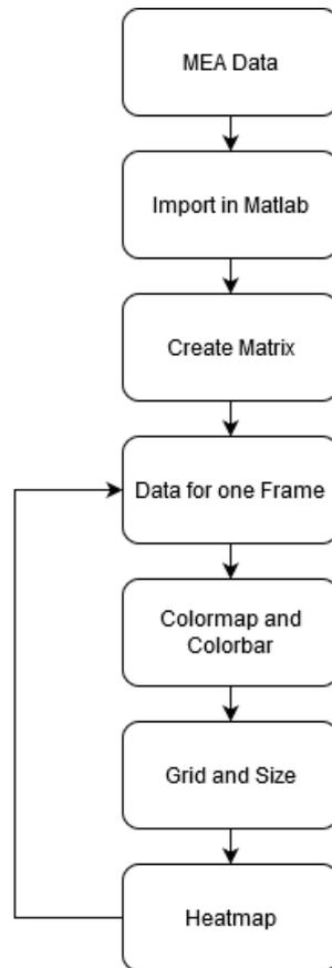
Figure 3.6: Flowchart describes the code to create the heatmap in Matlab, for CMOS-MEA and 60 electrode MEA files For the 60 electrode chip device small adjustments were done.
