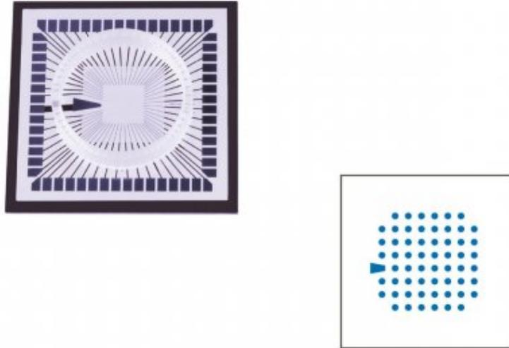
Figure 1.9: MEA chip with 60 electrodes, on the left side the chip on the right side the schematic electrodes. [29]
