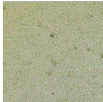
Figure 4.11: Image show the resized MEA array with dissociated neurons on it.
