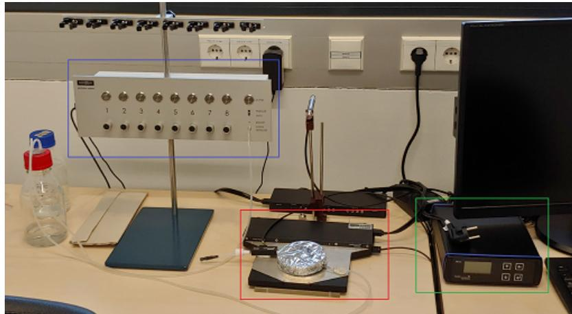
Figure 3.2: Measurement setup with the important devices showing headstage in red, temperature controller in green, perfusion and vacuum system in blue
