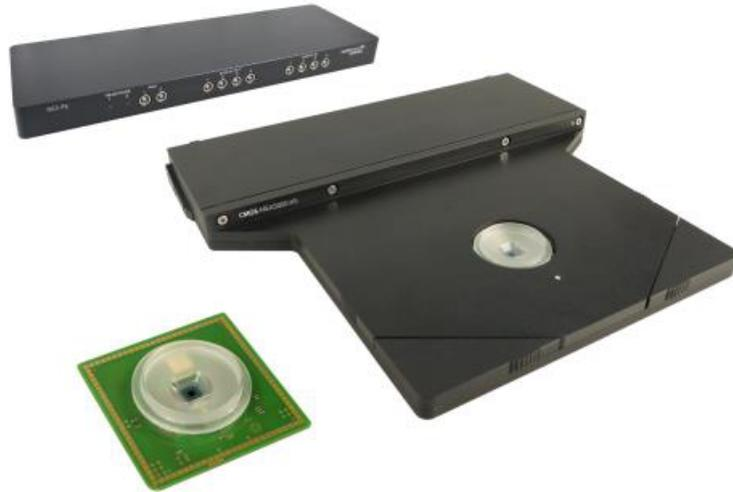
Figure 1.7: MEA-5000 system with headstage, interface board and MEA chip. [16]
