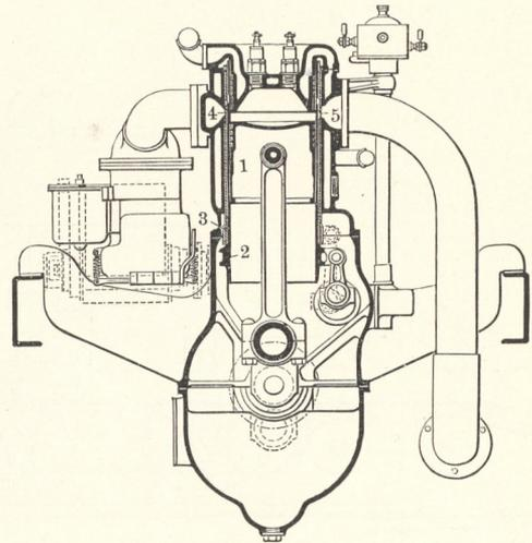
Fig. 263. Knightmaschine.
