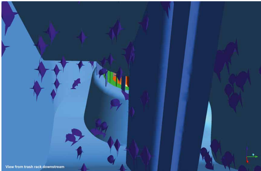
Figure 2: Numerical simulation of downstream fish migration.
