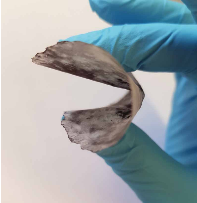
Figure 1: Chitosan anion exchange membrane doped with graphene oxide for use in direct alkaline alcohol fuels.
