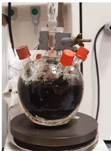
Figure 3: Synthesis of corrosion-resistant carbon supported catalyst for PEM fuel cell electrodes.
