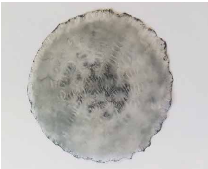
Figure 1: Chitosan anion exchange membrane doped with graphene oxide for use in direct alkaline alcohol fuels.
