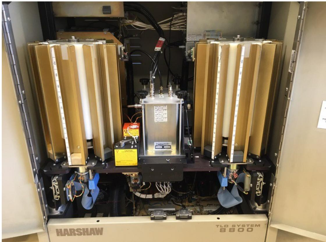
Figure 9: TLD Reader 8800 with four photomultipliers, heater nozzles, heating tube, depots for TLD cards and internal irradiation source.
