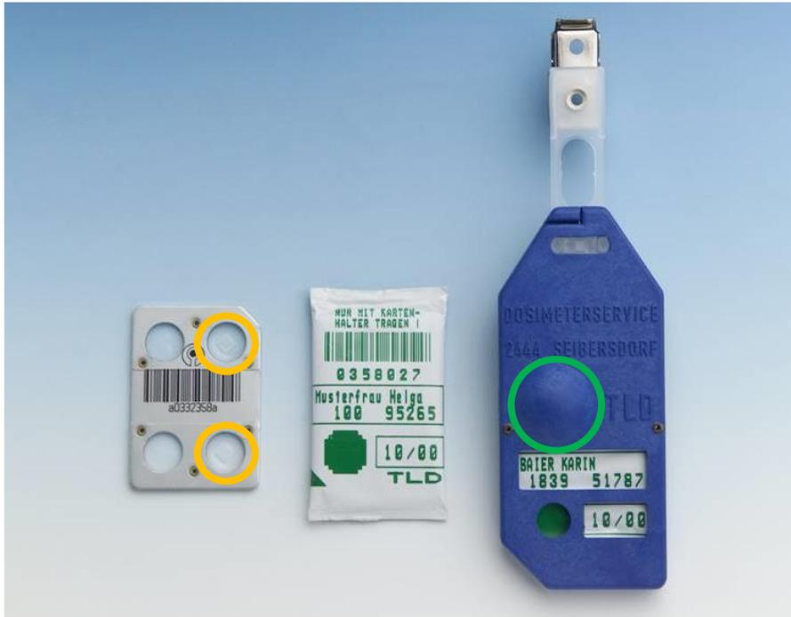
Figure 8: On the left side a TLD-100 card with two LiF:Mg,Ti chips encased in Teflon™ (orange circles) is shown. A sealed card for the customer is depicted in the middle. On the right side the card is placed in a badge. In the green circle there is an aluminium disc which shields one of the two elements. ©Seibersdorf Laboratories
