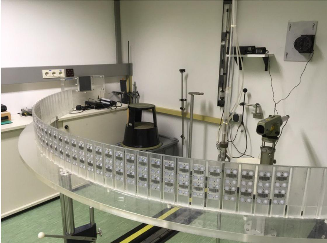
Figure 13: Panoramic irradiation facility (PIF): TLD cards are placed in the circular segment stand. The irradiation source is injected through the transparent pipe. An ionising chamber is placed near the source to measure the dose rate.
