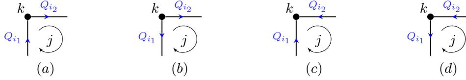
FIGURE A.1: Cases of different directions of flows  $Q_{i_1}$  and  $Q_{i_2}$  of node  $k$  which is also part of loop  $j$ .
