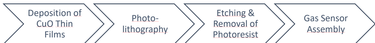
Scheme 1: Overview of experimental steps ranging from thin film deposition up to the final gas sensor.
