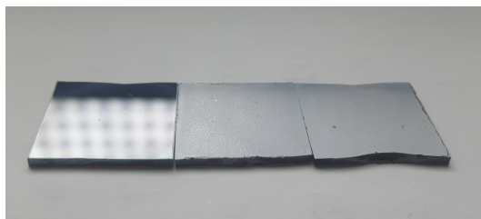
Figure 3.4: Difference in surface roughness for perovskite films fabricated using different amounts of anti-solvent. Photo shows perovskite films on glass substrates. Amount of applied anti-solvent (from left to right): 50 \mu\text{l} , 25 \mu\text{l} , 0 \mu\text{l} .
