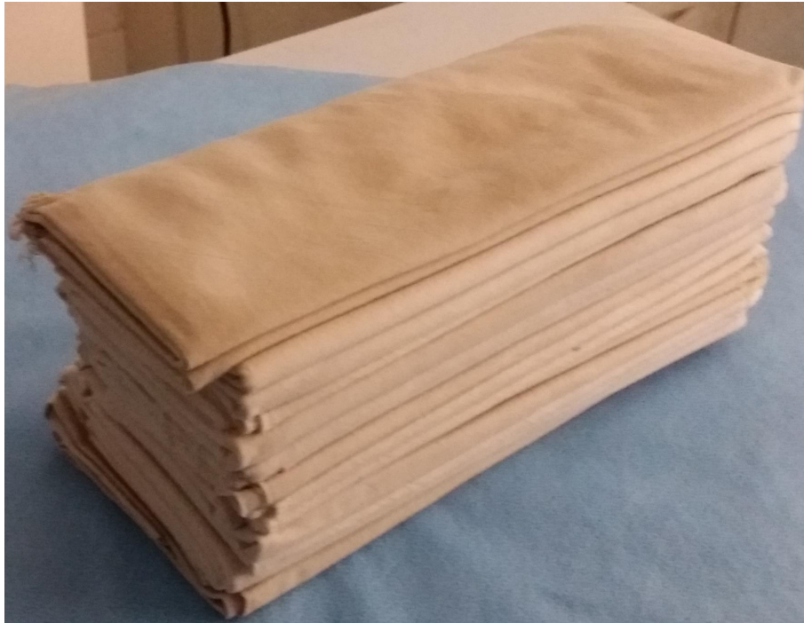
Figure 2.9: Picture of towels as an example of a porous load.
