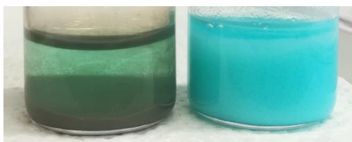
Figure 41 Copper nitrate/NDC-Na after 6 hours of storage at 80°C (left) and room temperature (right)
