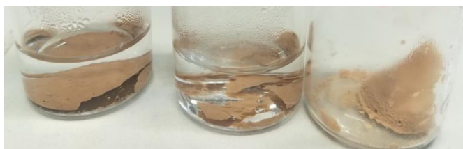
Figure 33 Formation of plates upon combination of NDC and manganese carbonate in different ratios (linker:metal) – left: 1:5, middle: 1:1, right: 1:1.33
