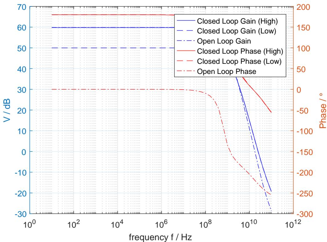
FIGURE 4.4: Bode plot of a 2 step variable gain amplifier
