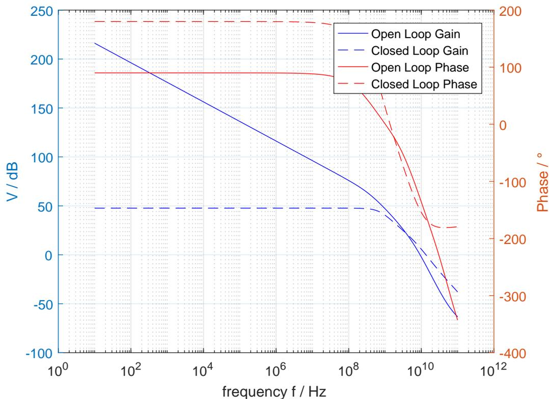
FIGURE 2.10: Bode plot of a three stage inverter amplifier.
