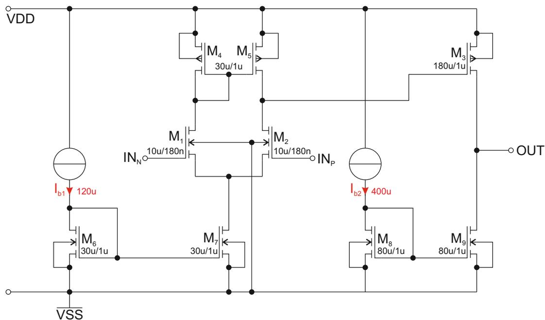
FIGURE 4.3: Dimensioning of a comparator.
