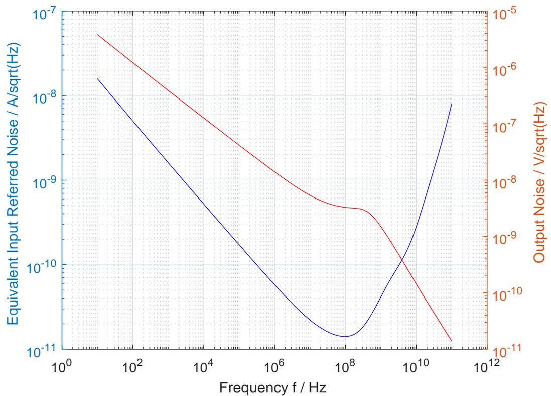
FIGURE 2.12: Noise analysis of a three stage inverter amplifier.
