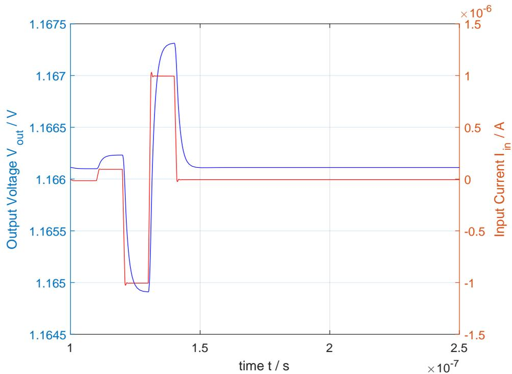
FIGURE 2.19: Transient response of a regulated cascode transimpedance amplifier with current mirrors.
