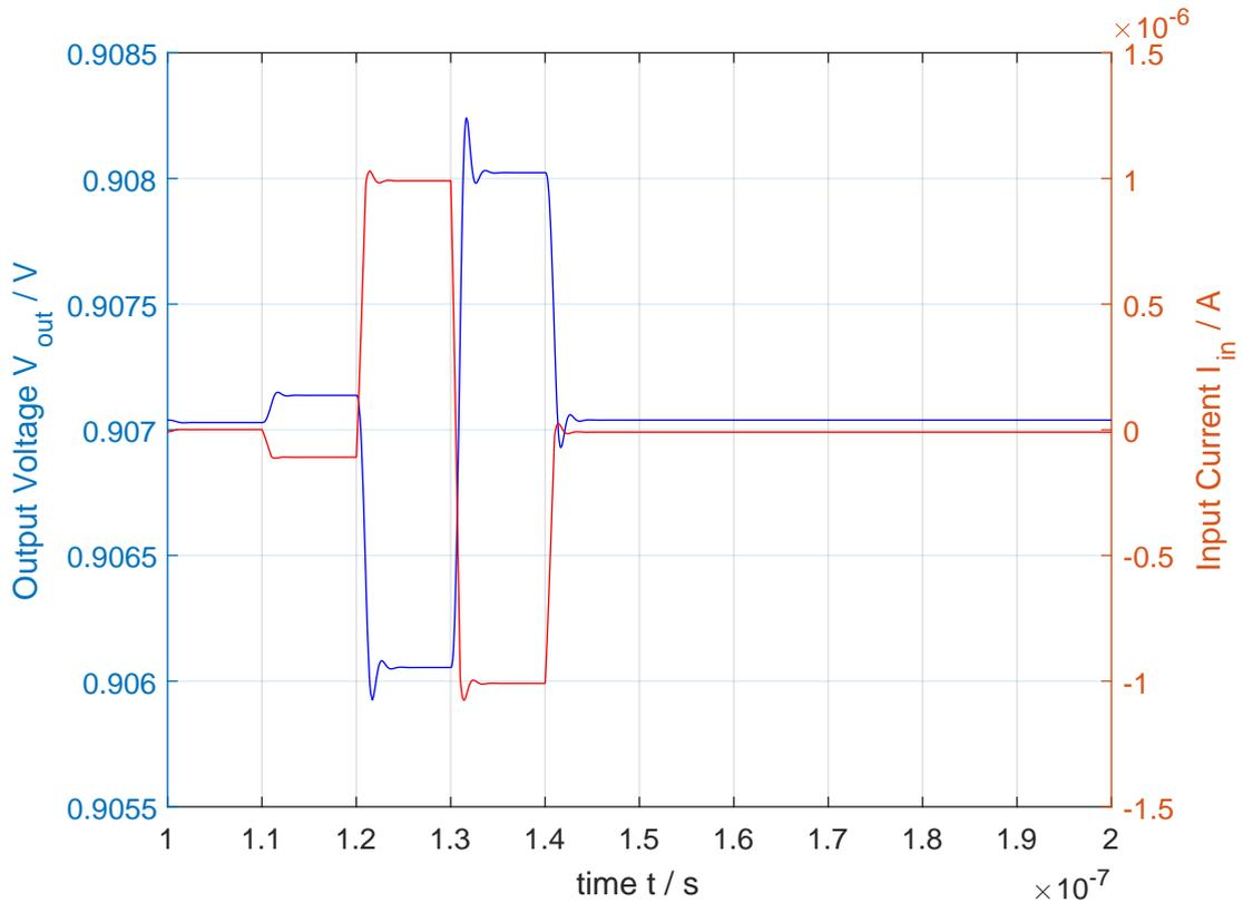
FIGURE 2.7: Transient response of a single stage push pull inverter based transimpedance amplifier with cascode.
