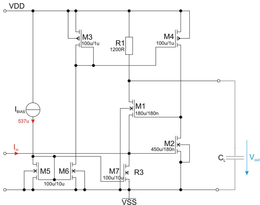
FIGURE 2.17: Schematic diagram of a regulated cascode transimpedance amplifier with current mirrors.
