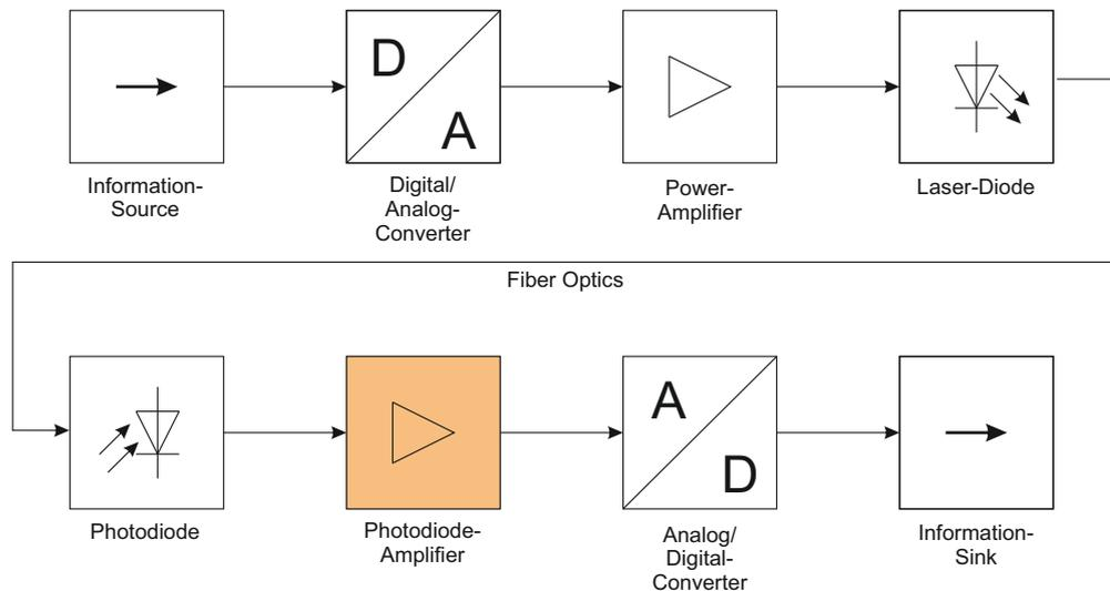
FIGURE 1.4: Structure diagram of an optical transmission system.
