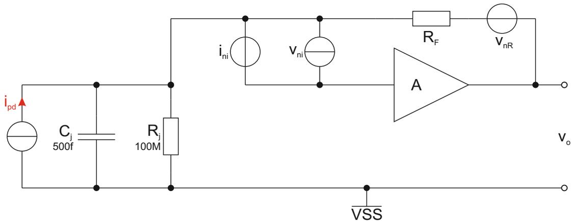
FIGURE 1.5: Noise analysis model of a basic photodiode amplifier.
