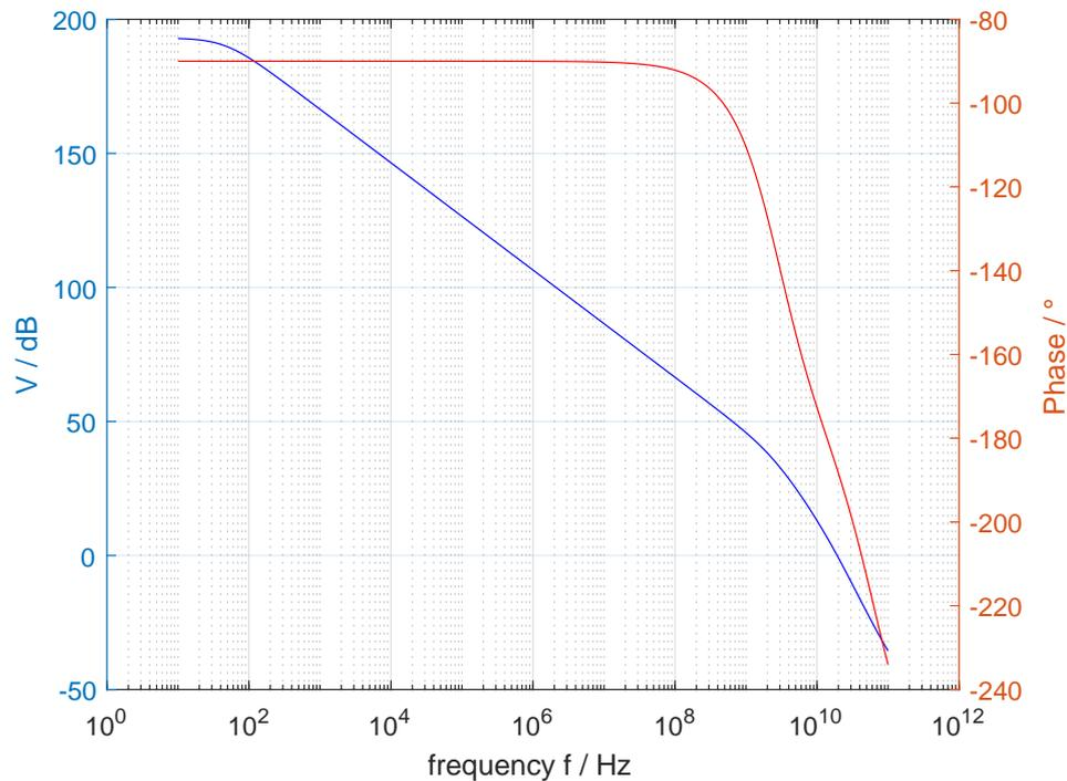
FIGURE 2.2: Open loop Bode diagram of the single stage inverter TIA
