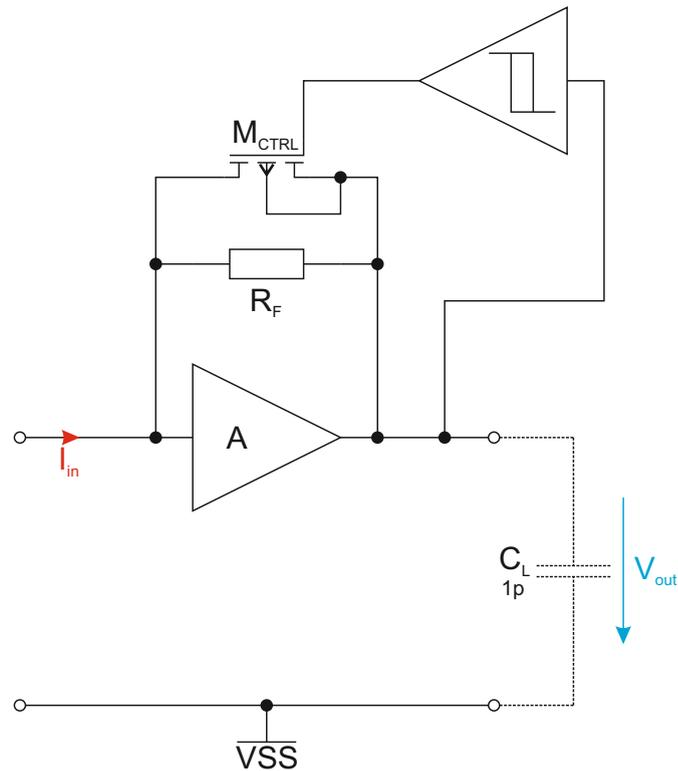
FIGURE 4.1: Toplevel circuit diagram of the proposed adjustable gain amplifier consisting of a conventional transimpedance amplifier, a comparator and an adjustable feedback network.
