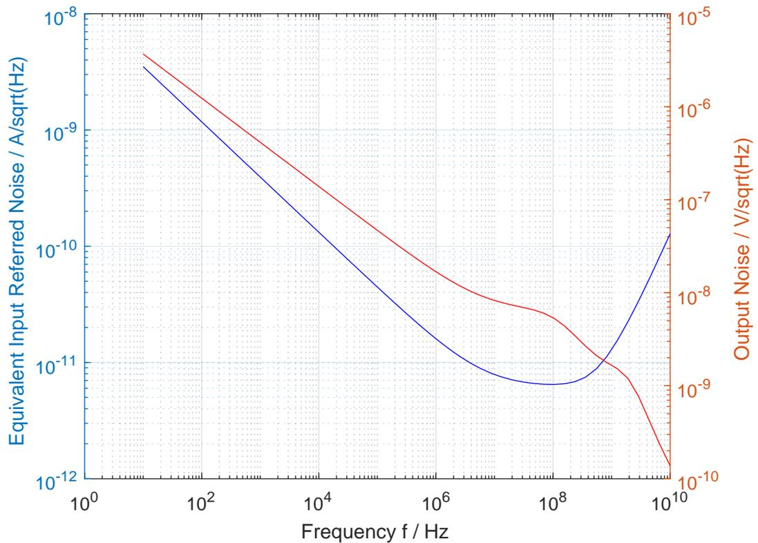
FIGURE 2.16: Noise behaviour of a regulated cascode TIA with resistors.
