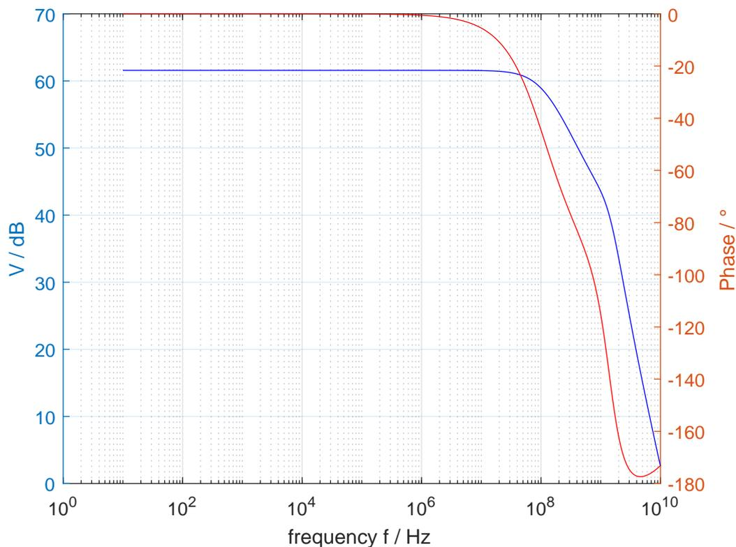
FIGURE 2.18: Closed loop Bode plot of a regulated cascode transimpedance amplifier with current mirrors
