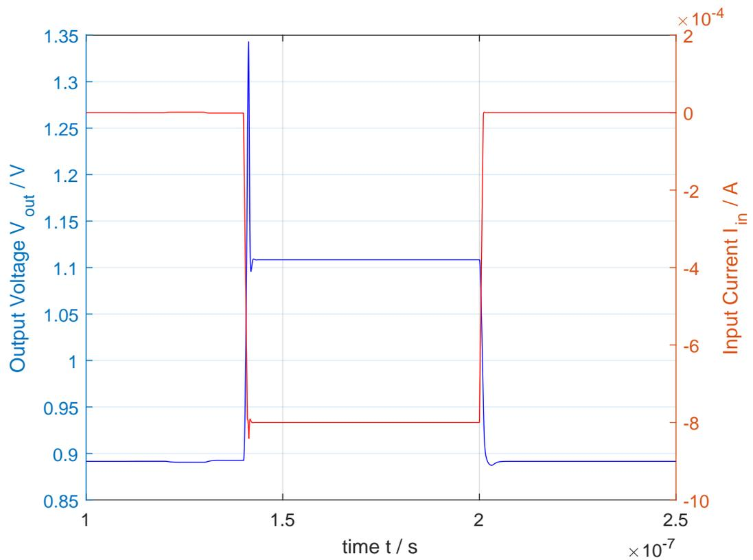
FIGURE 4.5: Transient response a 2 step variable gain amplifier
