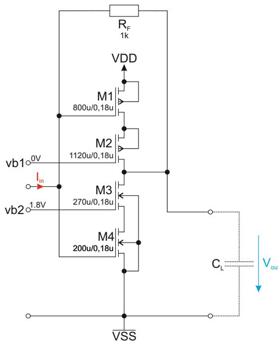
FIGURE 2.5: Schematic of a transimpedance amplifier based on a single stage cascoded push-pull inverter with feedback resistor  $R_F$  and load capacitance  $C_L$  and a diode load after each stage.
