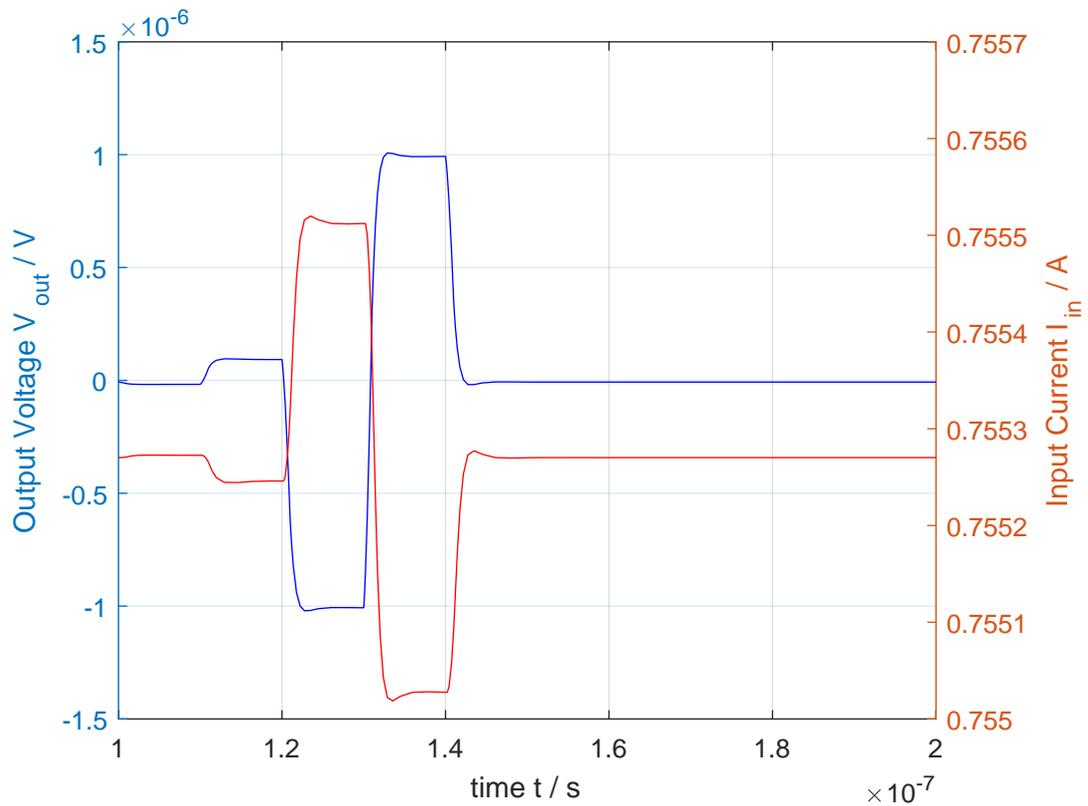
FIGURE 2.11: Transient analysis of a three stage inverter amplifier.
