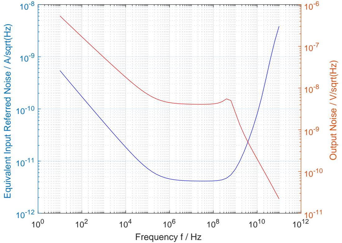
FIGURE 2.8: Noise analysis of a single stage cascoded push-pull inverter based transimpedance amplifier. The blue curve shows input referred current noise, whereas the red curve shows the output noise voltage.
