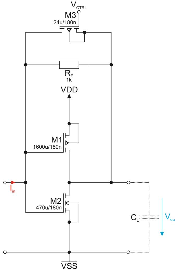
FIGURE 4.2: Dimensioning of 2 step automatic gain TIA.
