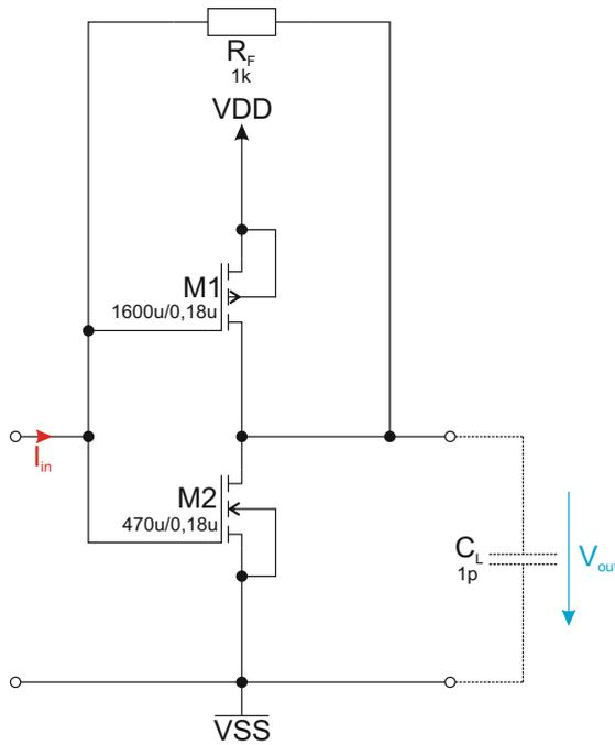
FIGURE 2.1: Schematic of a single stage inverter transimpedance amplifier with feedback resistor  $R_F$  and load capacitance  $C_L$ .
