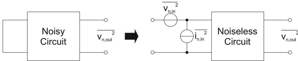
FIGURE 1.7: Conversion between measurable output noise  $\overline{v_{n,out}^2}$  and the theoretical, though often used input referred noise sources  $\overline{v_{n,in}^2}$  and  $\overline{i_{n,in}^2}$ .
