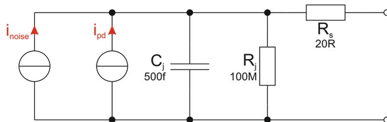
FIGURE 1.3: Equivalent circuit diagram of a photodiode.
