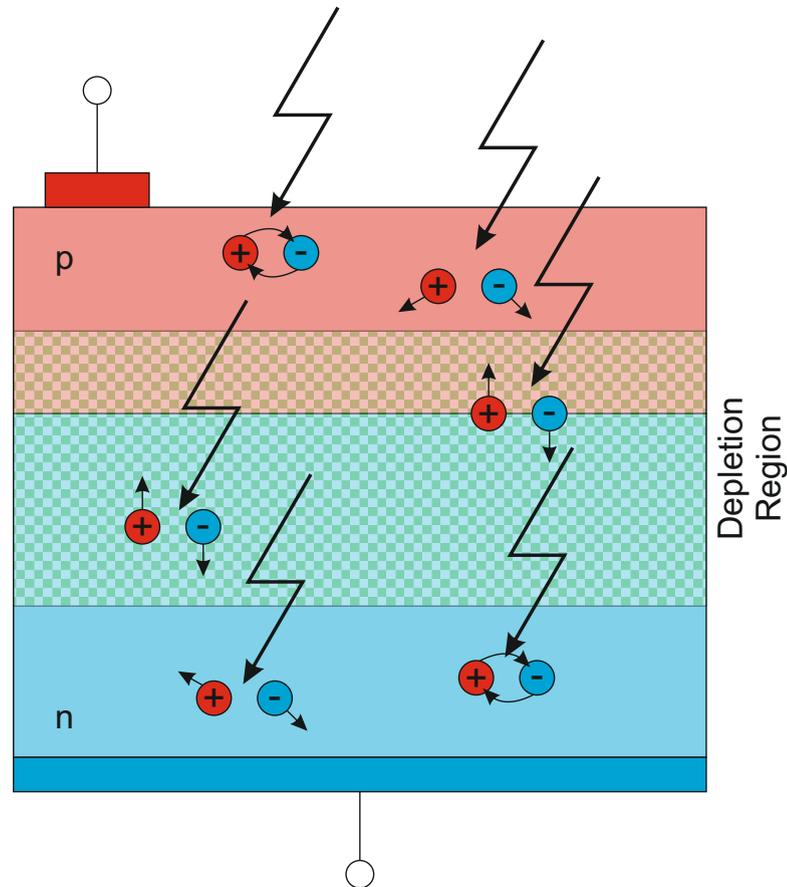
FIGURE 1.2: In a photodiode, photons produce electron-hole pairs. Within the depletion region they get separated and accelerated towards the terminals, whereas the electron-hole pairs occurring outside the depletion region either recombine immediately or travel by diffusion.
