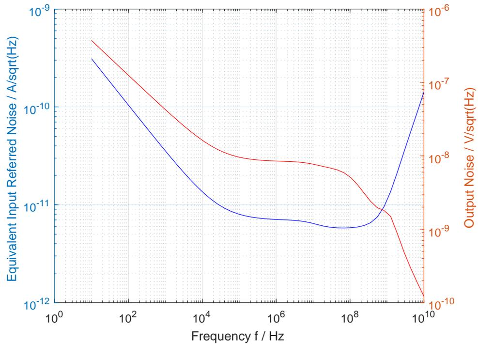
FIGURE 2.20: Noise figure of a regulated cascode transimpedance amplifier with current mirrors.
