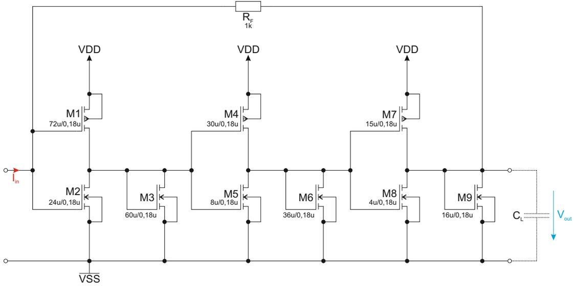
FIGURE 2.9: Schematic of a three stage inverter transimpedance amplifier with feedback resistor  $R_F$  and load capacitance  $C_L$  and a diode load after each stage. At the first stage a cascode circuit is used to increase the gain, and thus the noise figure of the circuit.
