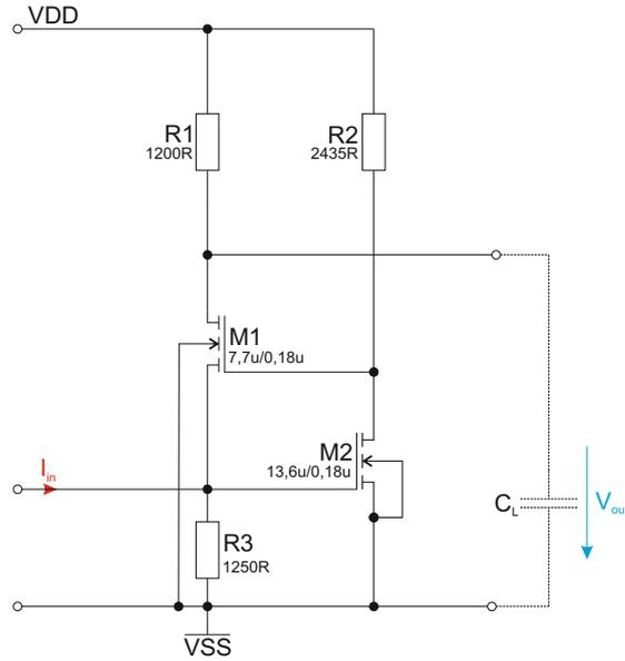
FIGURE 2.13: Circuit diagram of a regulated cascode TIA with resistive biasing.
