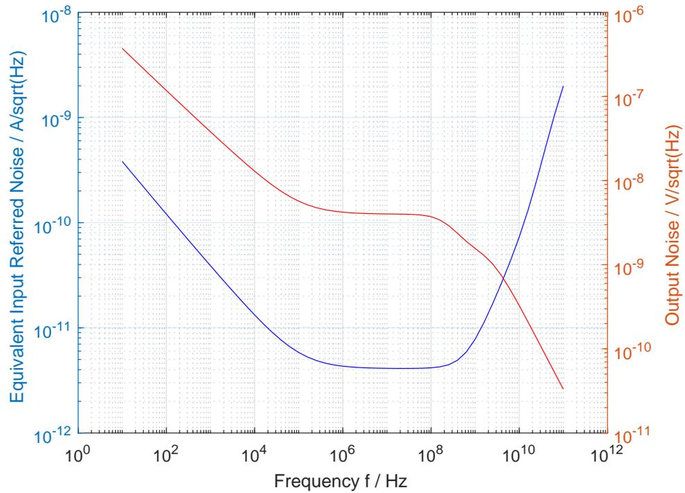
FIGURE 2.4: Noise analysis the proposed single stage push pull inverter transimpedance amplifier. The red line represents the noise voltage at the output, whereas the blue line represents the equivalent input referred noise current.
