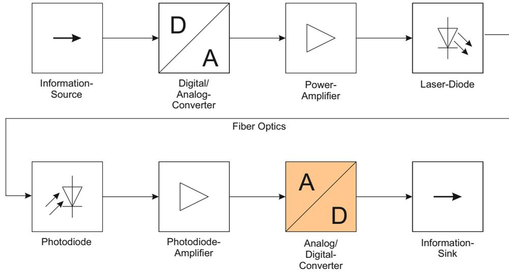
FIGURE 1.8: Structure diagram of an optical transmission system.
