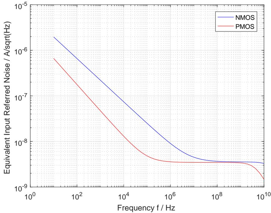
FIGURE 3.2: Comparison of input referred noise behaviour for NMOS and PMOS devices driving the same current.
