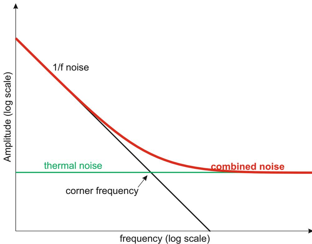
FIGURE 1.6: Power spectral densities of thermal and flicker noise at a MOSFET. The flicker noise dominates the low frequency section whereas the thermal noise dominates at higher frequencies.
