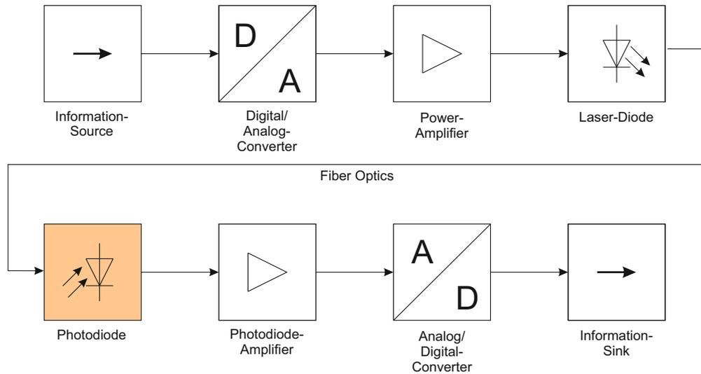
FIGURE 1.1: Structure diagram of an optical transmission system.
