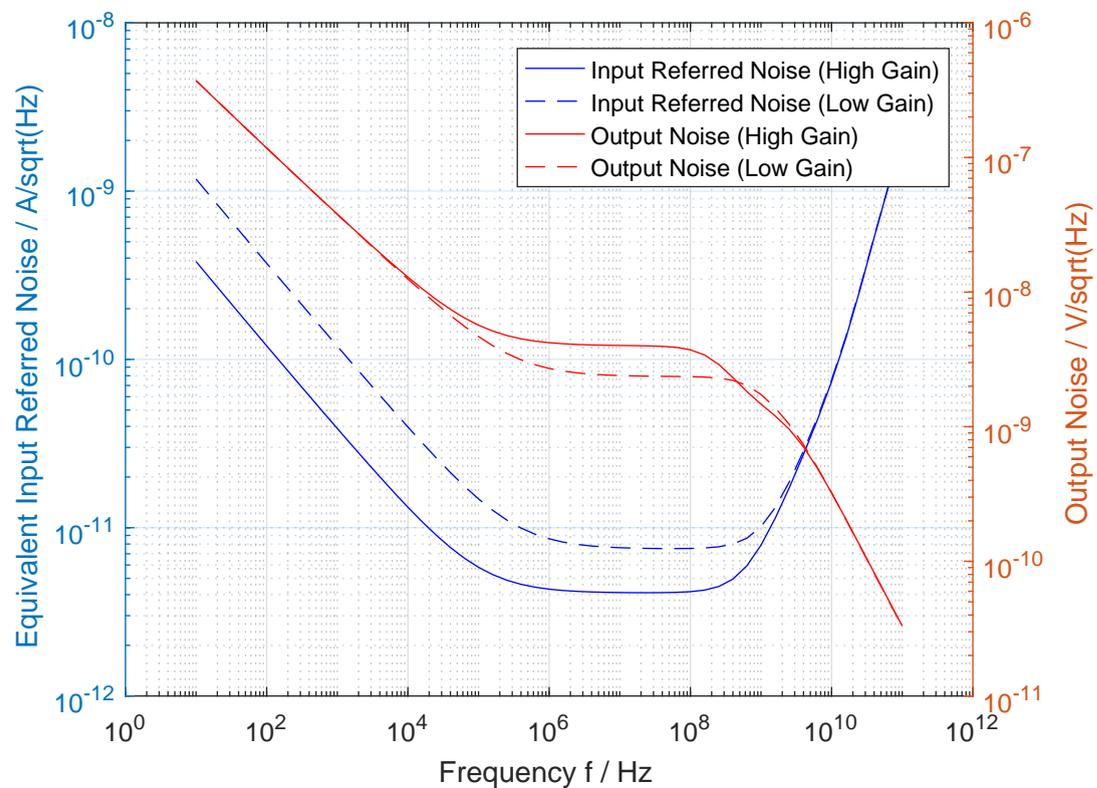
FIGURE 4.6: Noise response of a 2 step variable gain amplifier
