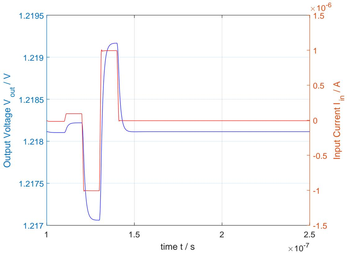
FIGURE 2.15: Transient response of a regulated cascode TIA with resistive biasing.
