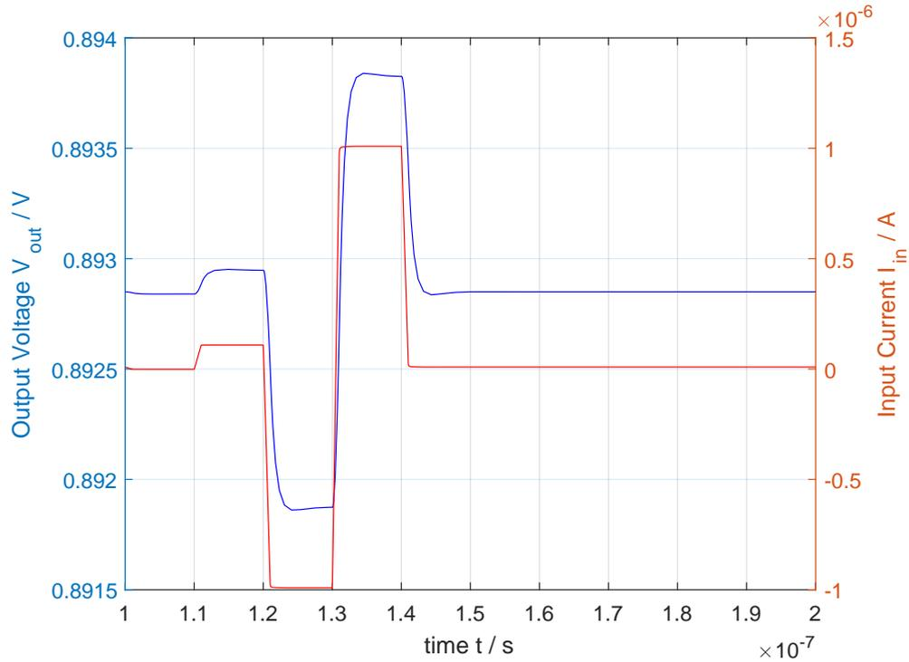
FIGURE 2.3: Transient analysis the proposed single stage push pull inverter transimpedance amplifier. There can be a little overshoot observed at the edges, but it is still considered to be stable.
