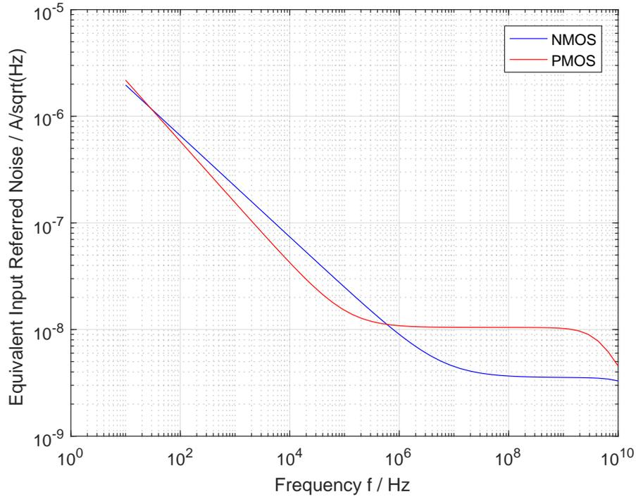
FIGURE 3.1: Comparison of input referred noise behaviour of same sized NMOS and PMOS transistors. The width of both transistors is set to  $W = 20 \mu\text{m}$
