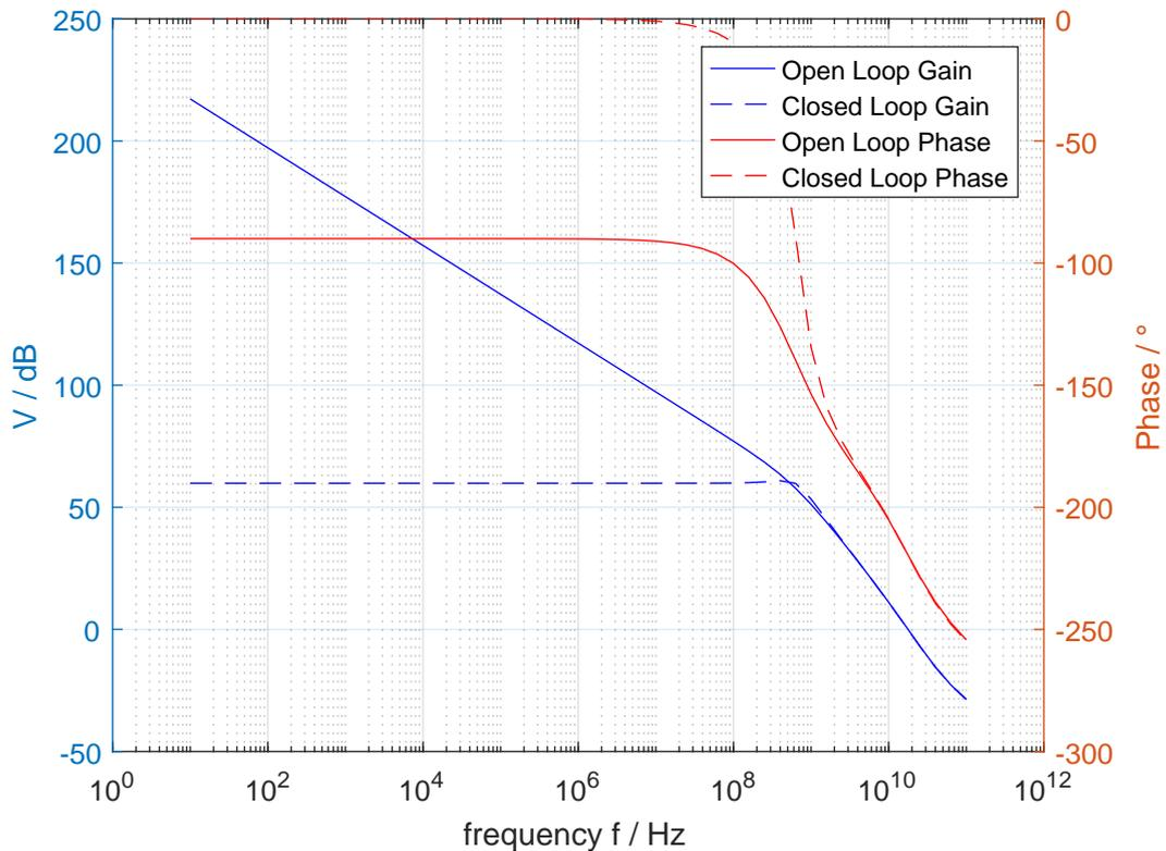
FIGURE 2.6: Bode plot of a single stage inverter amplifier with cascode. The solid line depicts the open loop configuration, whereas the dashed line represents the closed loop configuration with a feedback resistance of  $R_F = 1 \text{ k}\Omega$ .
