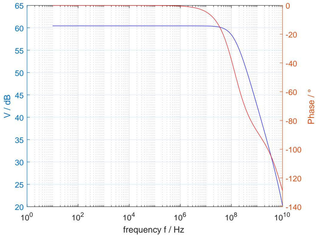
FIGURE 2.14: Bode plot of a regulated cascode TIA with resistors
