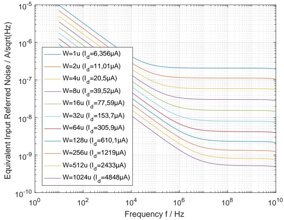
FIGURE 3.3: Comparison of input referred noise behaviour for different sized NMOS transistors and different currents. The gate voltage  $V_G$  is kept constant.
