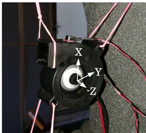
**Figure 5.5:** Measurement setup for the acceleration measurements.
