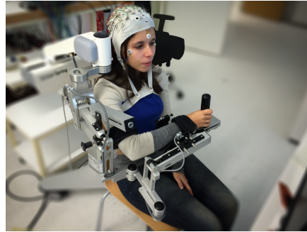
Fig. 2: A subject mounted with the electrode cap and the Armeo exoskeleton.
