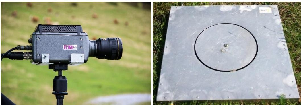
Figure 6: High speed video camera (left) and flat plate antenna (right)
