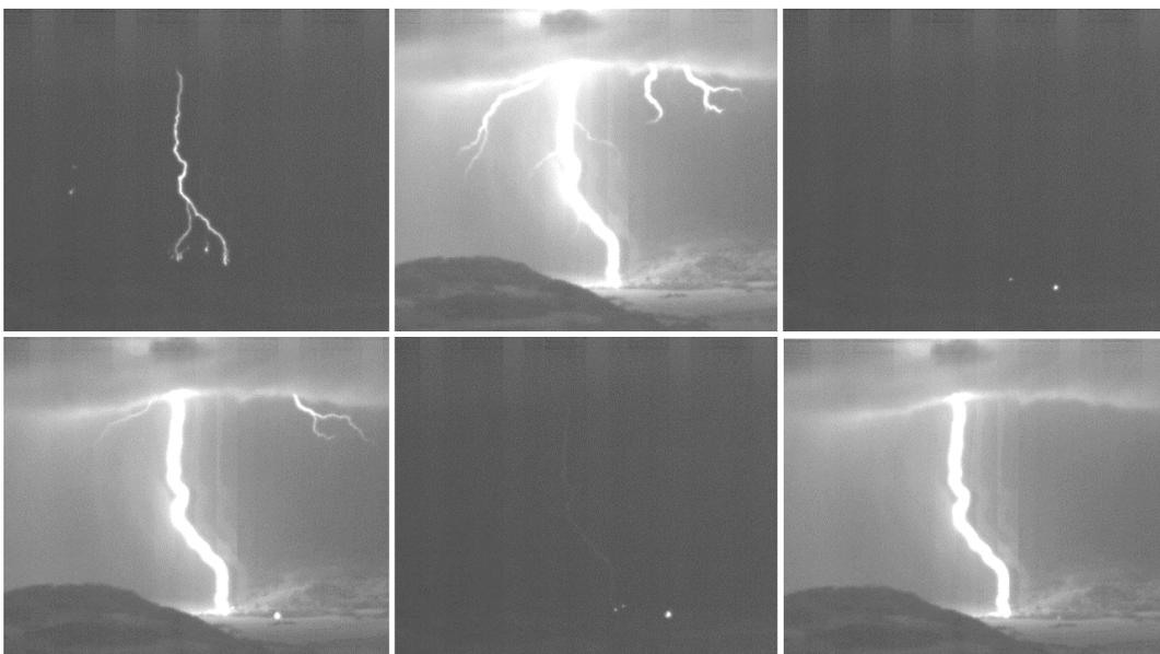
Figure 32: Stepped leader, first return stroke (F11), flashover on two towers, subsequent stroke 2 (SU1), flashover on three towers and subsequent stroke 3 (SU1) from top left to bottom right
