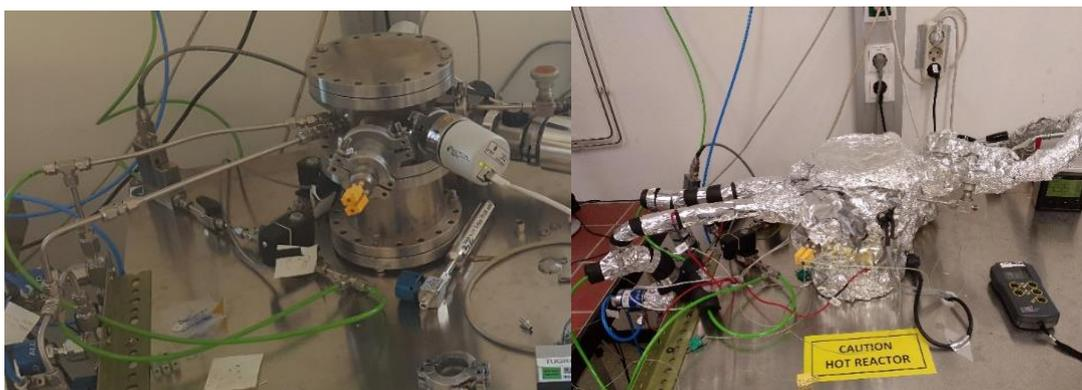
Figure 27: MLD system before and after thermal isolation
