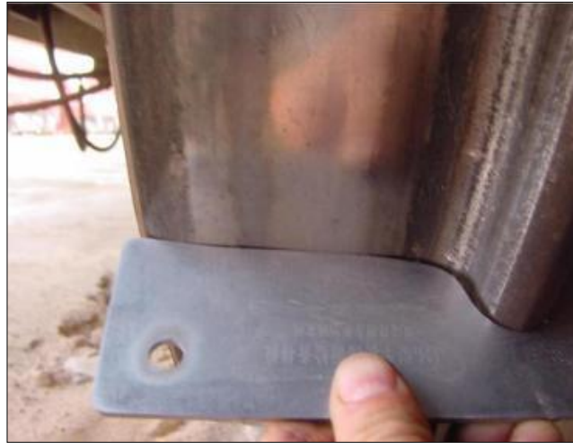
Figure 45: Worn wheel profile compared with a new profile shape on a metal gauge 82
