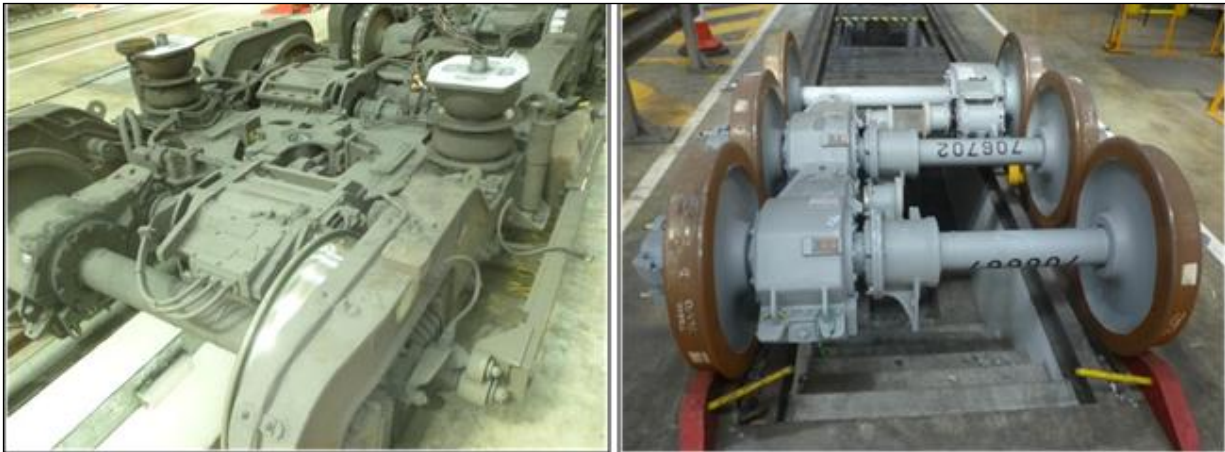
Figure 39: Jubilee line bogie and its wheelset
