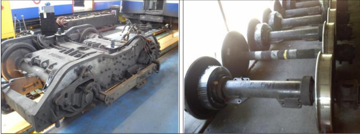
Figure 37: Bogie of Bakerloo line and semi suspended wheelset concept
