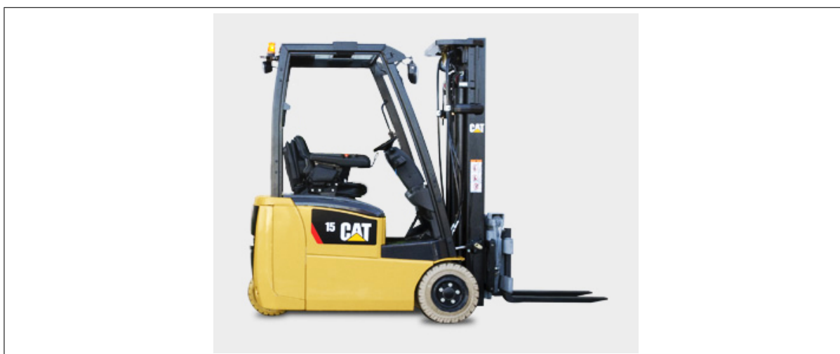
Figure 5.6: 3-wheel 48 V forklift truck. 267
