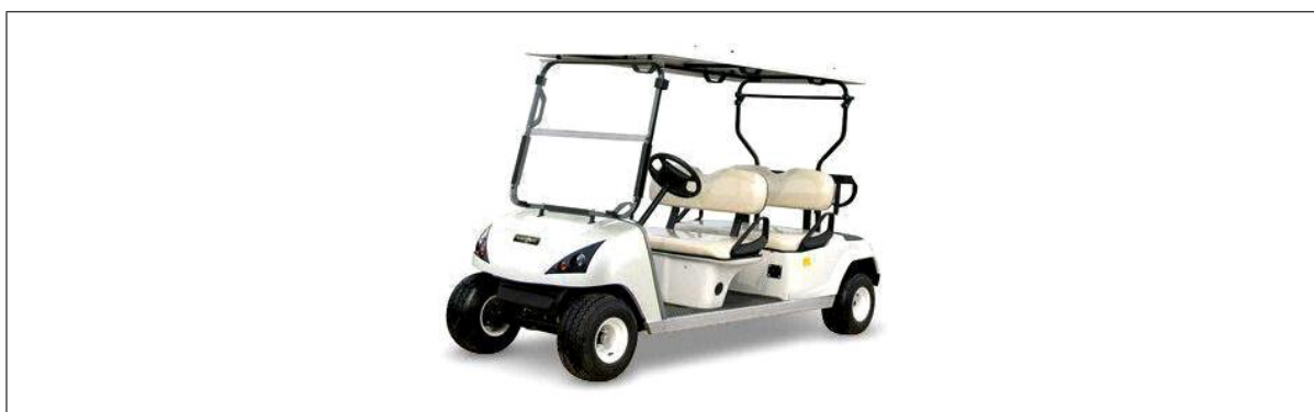
Figure 5.7: A golf cart with a 48 V motor supplied by six batteries of 8 V. 272
