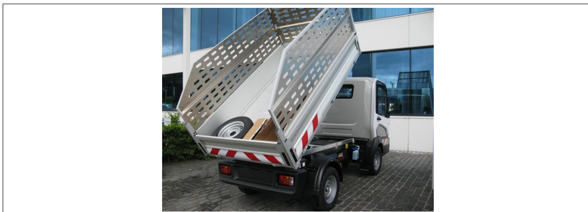
Figure 5.9: Goupil G5-E Van & Tipper with a 48 V system voltage. 278
