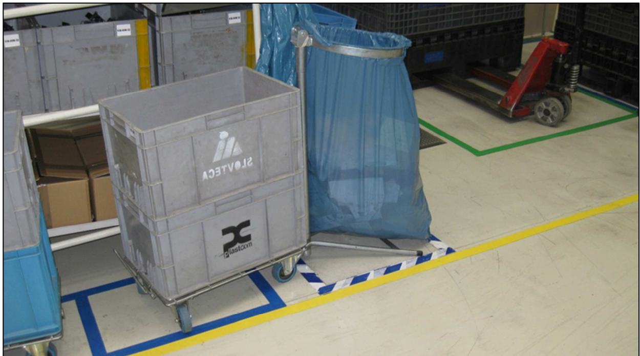
Figure 15: Colored floor markings at Magna Slovteca 165
