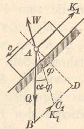
$\sphericalangle BAC_1 = \alpha - \varphi; \sphericalangle BC_1A = 90^\circ + \varphi,$
