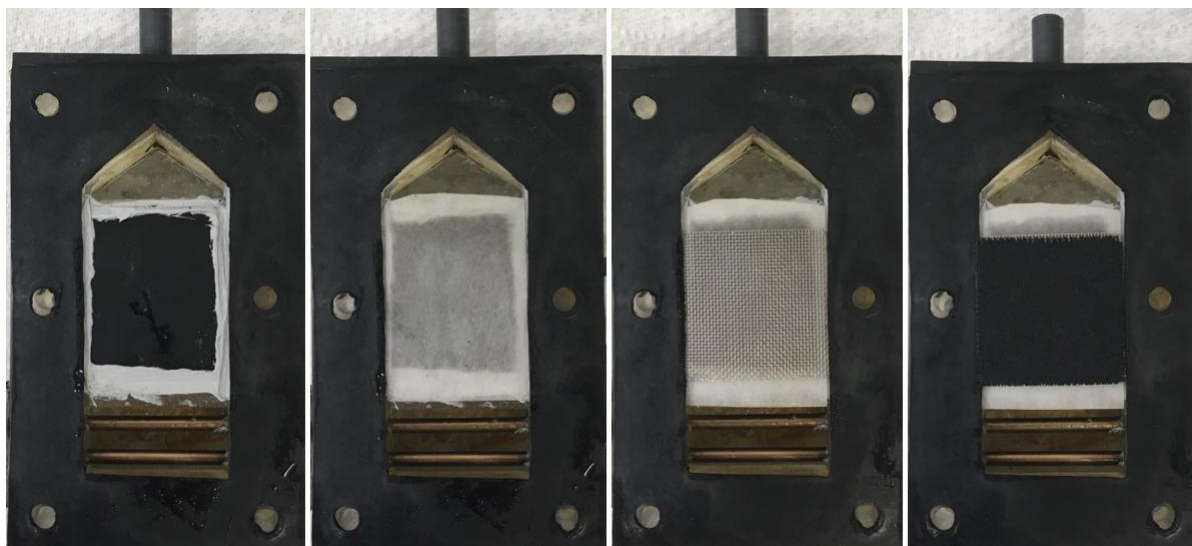
Figure 3-1: Cell assembly process from left to right: gluing in the cathode, applying the separator, the Ni mesh and the anode.
