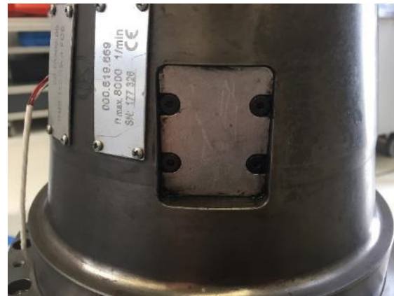
Figure 42: Kessler spindle with preliminary space to implement an accelerometer
