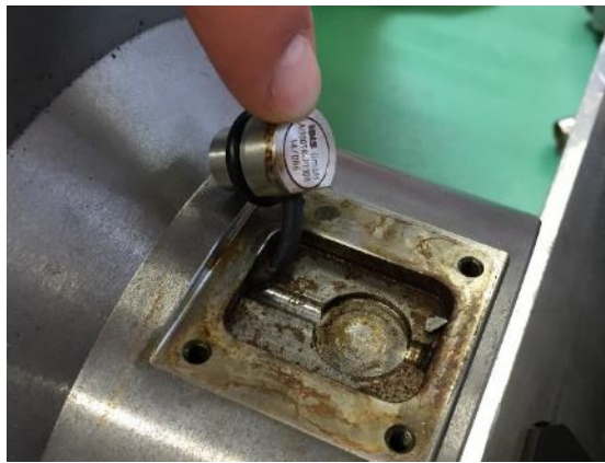
Figure 41: Corcom spindle with integrated IBIS accelerometer
