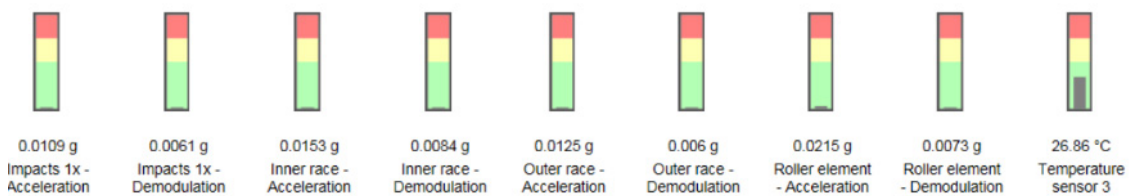
Figure 89: SmartCheck - Status of all elements of a rolling bearing
