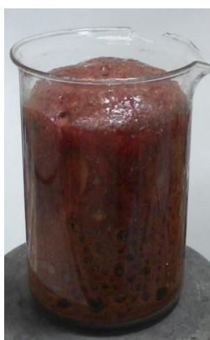
Fig. 13: Foaming of the Fe-based perovskite catalyst during the gelation process
