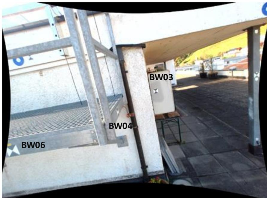
Figure 65: Targets BW03, BW04, and BW06 placed in the test field under different angles
