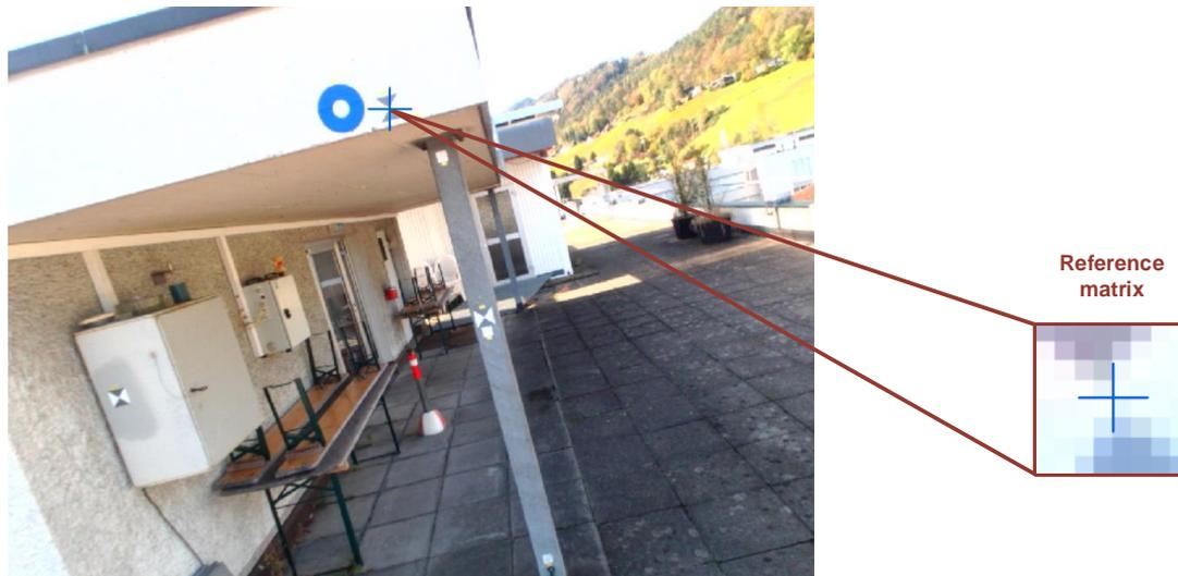
Figure 36: The reference matrix defined around the image point
