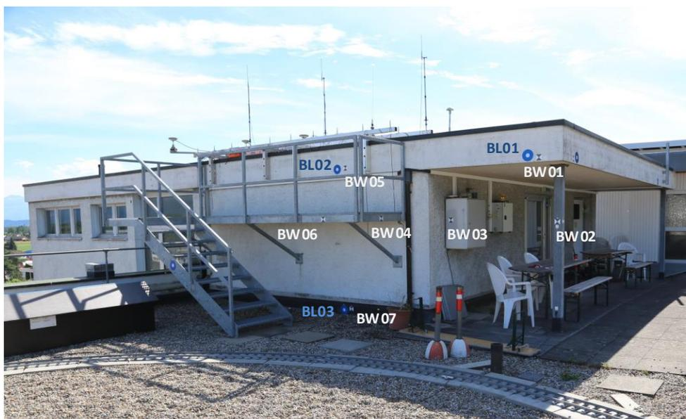
Figure 45: The blue and the black-and-white targets in the test field
