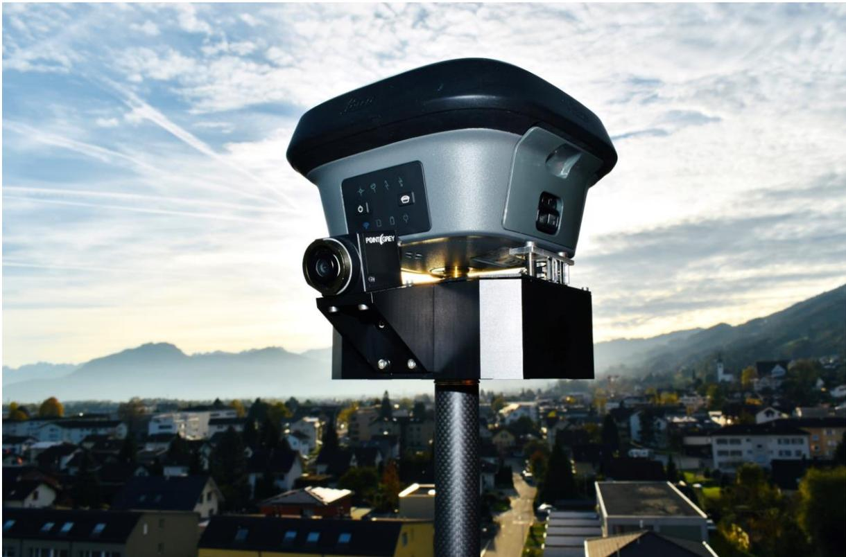
Figure 7: FuMo consisting of GNSS antenna and receiver, IMU and camera
