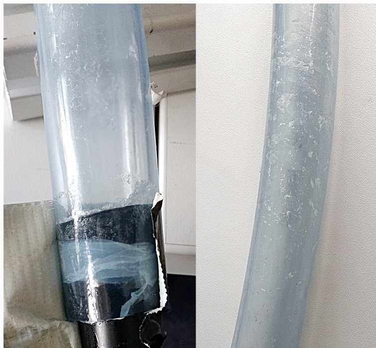
Figure 4.19: n -Eicosan is emitted by the L-Type HT-CPC during operation in large amounts. The working fluid partly condenses in the exhaust tube.
