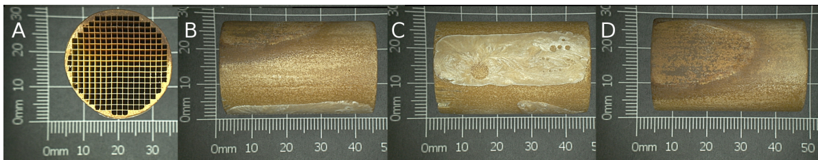
Figure 4.15: NGK cordierite ceramic after 18.25 h of use in setting 2: N_2 introduced at the carrier gas inlet. A) Front, B) side, C) bottom and D) top view.
