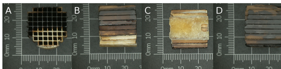
Figure 4.6: FRAUENTHAL HT ceramic after 18.25 h of use in setting 1: Unfiltered ambient lab air introduced at the carrier gas inlet. A) Front, B) side, C) bottom and D) top view.
