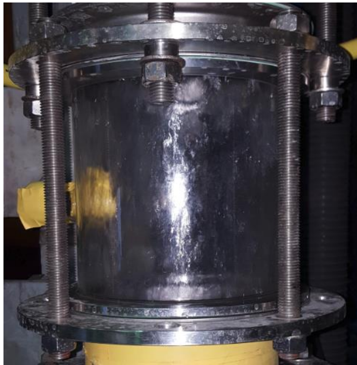
Figure 5-12: Flow of process water in the system; \Delta p \approx 0,16\text{bar} ; T \approx 55^\circ\text{C} ; \dot{V} \approx 5,7\text{m}^3/\text{min}
