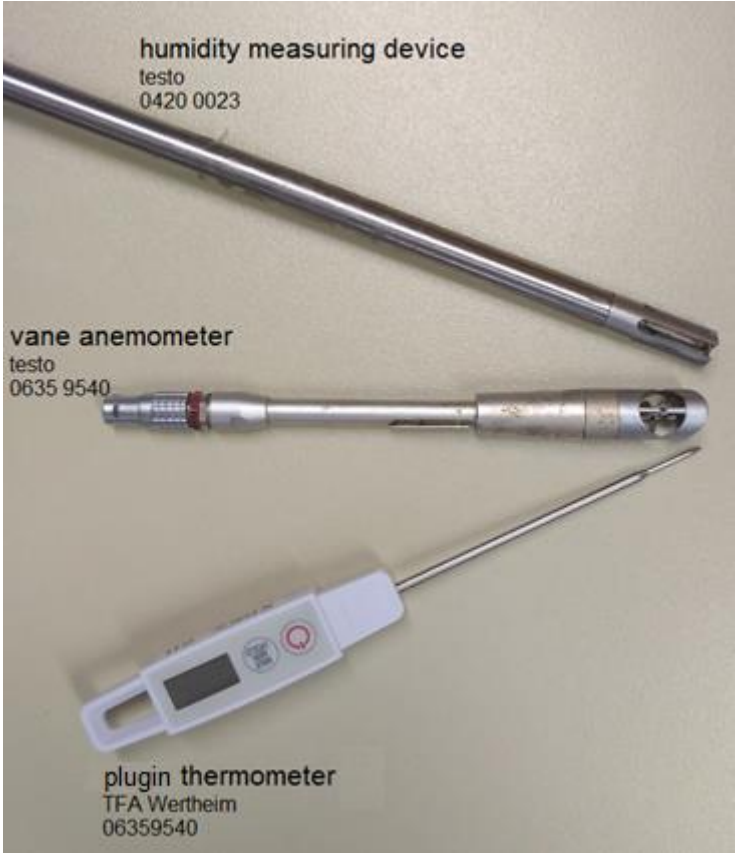
Figure 5-11: Measuring devices for verification of measurements
