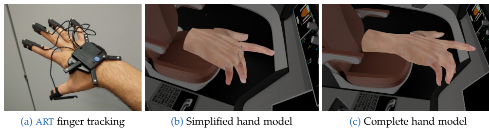
Figure 4.20.: The three types of hand and finger tracking representations.
