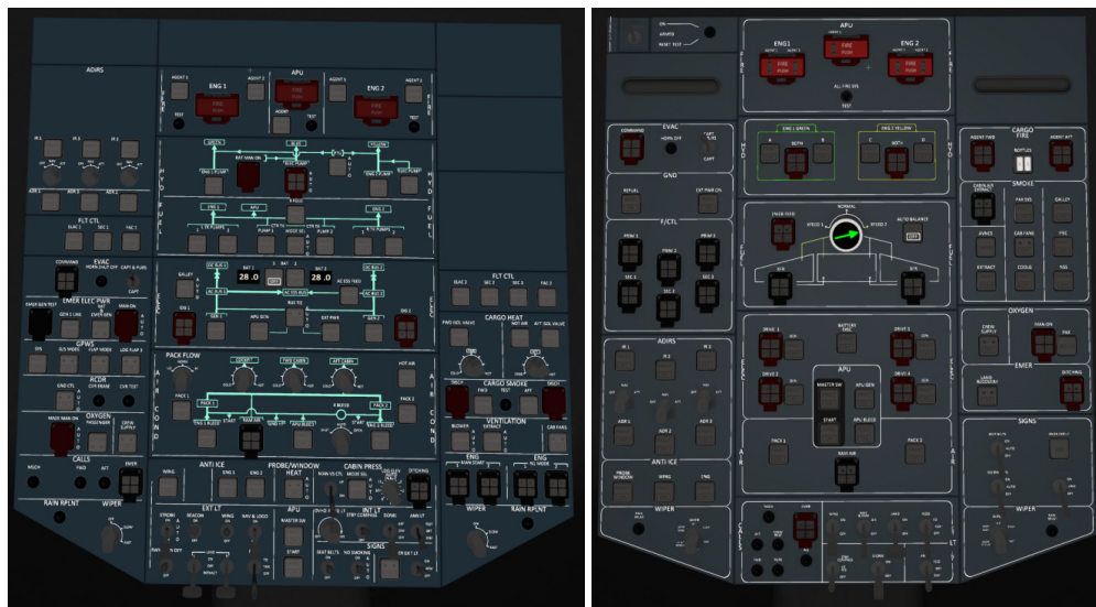
(a) The legacy overhead panel
