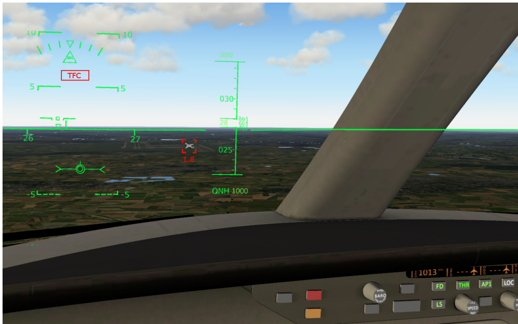
(b) The symbology of the head-worn device: The pilot is looking slightly to the right to fixate the other aircraft which already entered the non-transgression zone.
