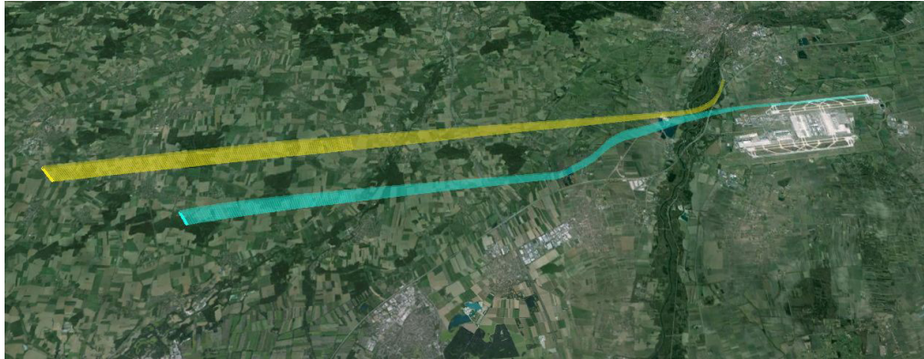
(a) The trajectory of the scenario: The yellow trajectory indicates the own aircraft; the cyan trajectory indicates the other aircraft with the late runway change.
