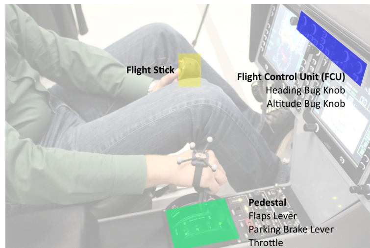
Figure 5.7.: Cockpit elements that are used for the simulator trial (Oberhauser, Dreyer, Braunstingl, et al., 2017b).
