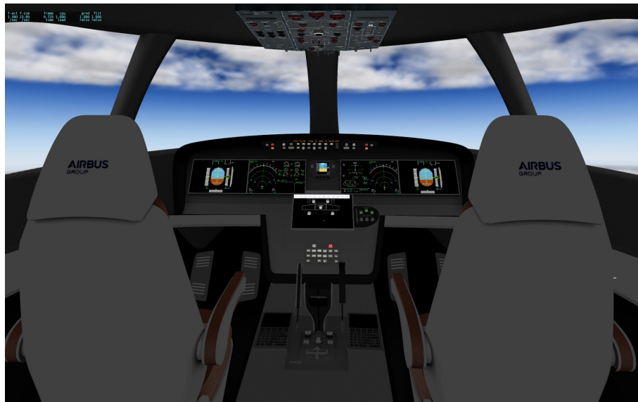
Figure 6.19.: The virtual cockpit with the overhead panel and the Soft-ICP in the central display of the cockpit.
