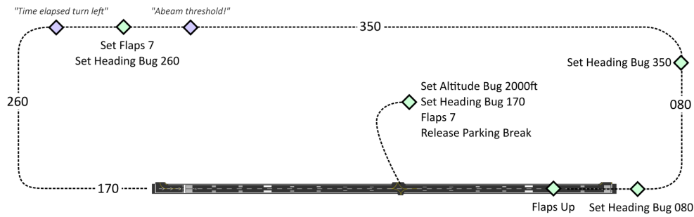
(a) The traffic circuit with the audio commands (Oberhauser, Dreyer, Braunstingl, et al., 2017b).
