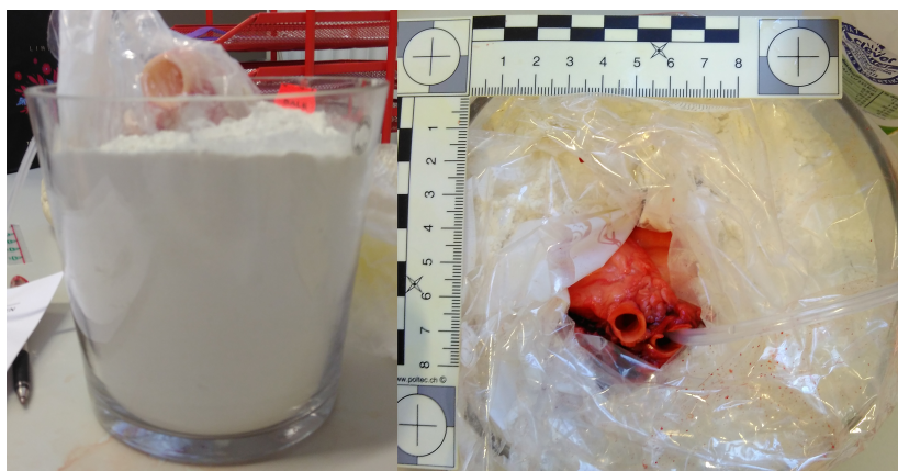
Figure 6.1: Example of experimental setup for MRI examination of ex situ porcine hearts. Flour was used to stabilise hearts for the duration of the examination.
