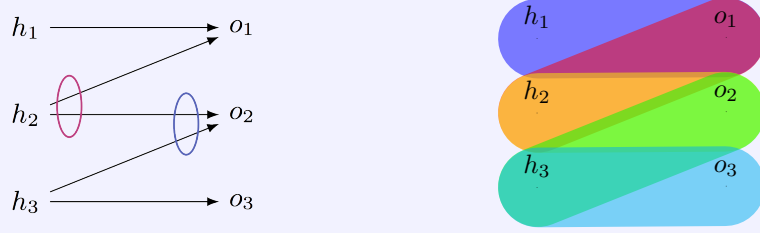
Figure 6.1: DAG and hypergraph representation. The DAG shows shared hypotheses (left oval) and common effects (right oval) for pairs of nodes.
