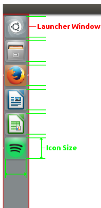
Figure 4.4: Ubuntu Unity application launcher. The geometry of the launcher window (red rectangle) can be retrieved from the operating system. The width is user configurable and the padding is fixed, therefore we use the width to calculate the height of the icons. With this information and the list of currently running applications we can calculate each individual application's launcher icon's geometry.
