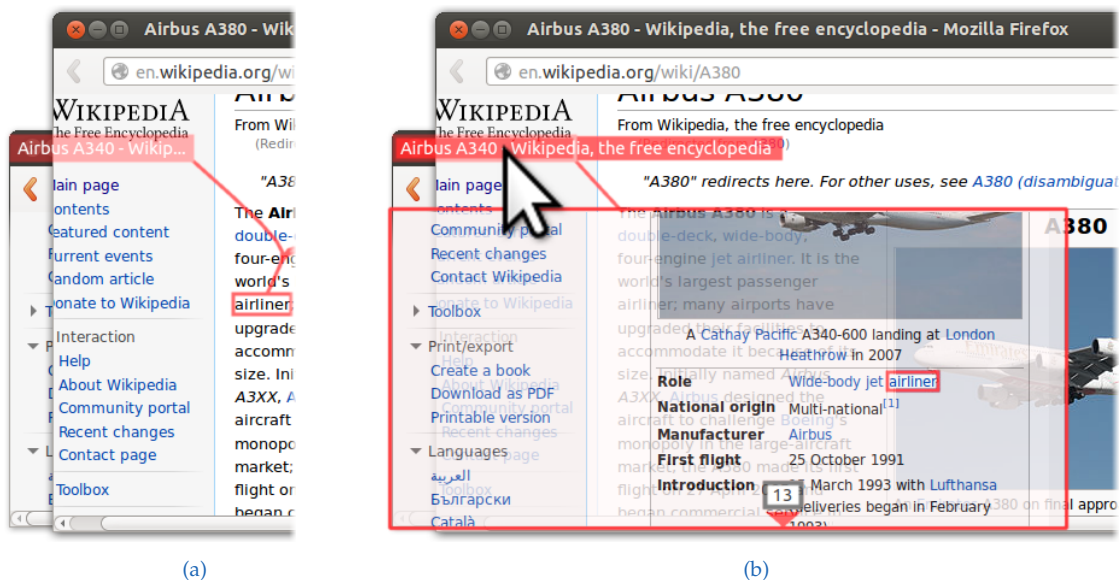
Figure 3.14: See-through visualization for occluded content. (a) A marker showing a part of the window title indicates occluded content. (b) On hovering over the marker covered content is superimposed, including highlights for the occluded content.
