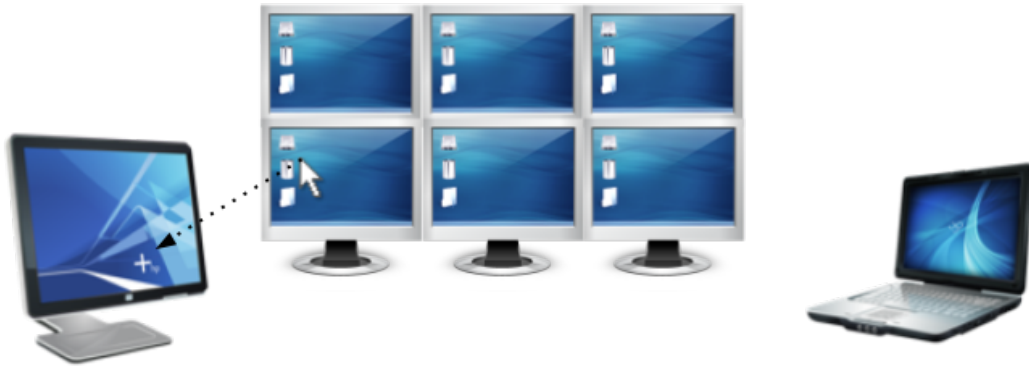
Figure 3.2: Example of an arrangement of two standard computers (left & right) and one computer with a large (six monitor) display (center) on an office table. Users can “teleport” with their mouse to each computer without changing the actual physical input devices.
