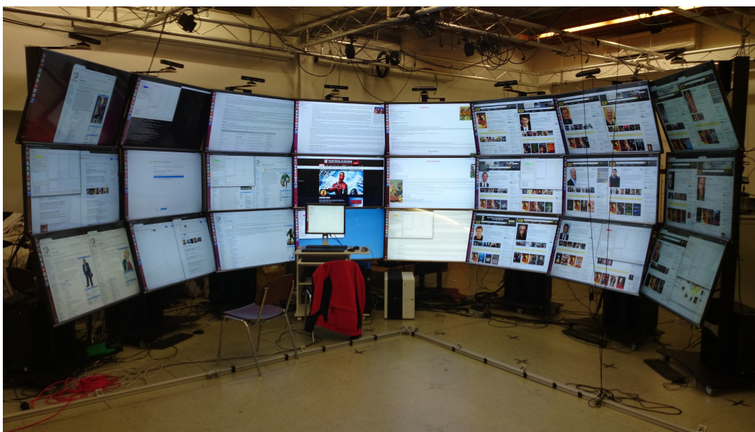
Figure 1.1: Our largest tiled display consists of 24 monitors (50", 1080p), arranged in a 8 \times 3 grid and driven by a cluster of eight computers.
