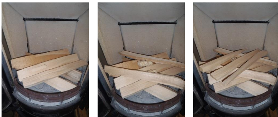
Figure 71: Lighting procedure of the ignition batch according to the top-down ignition technique
