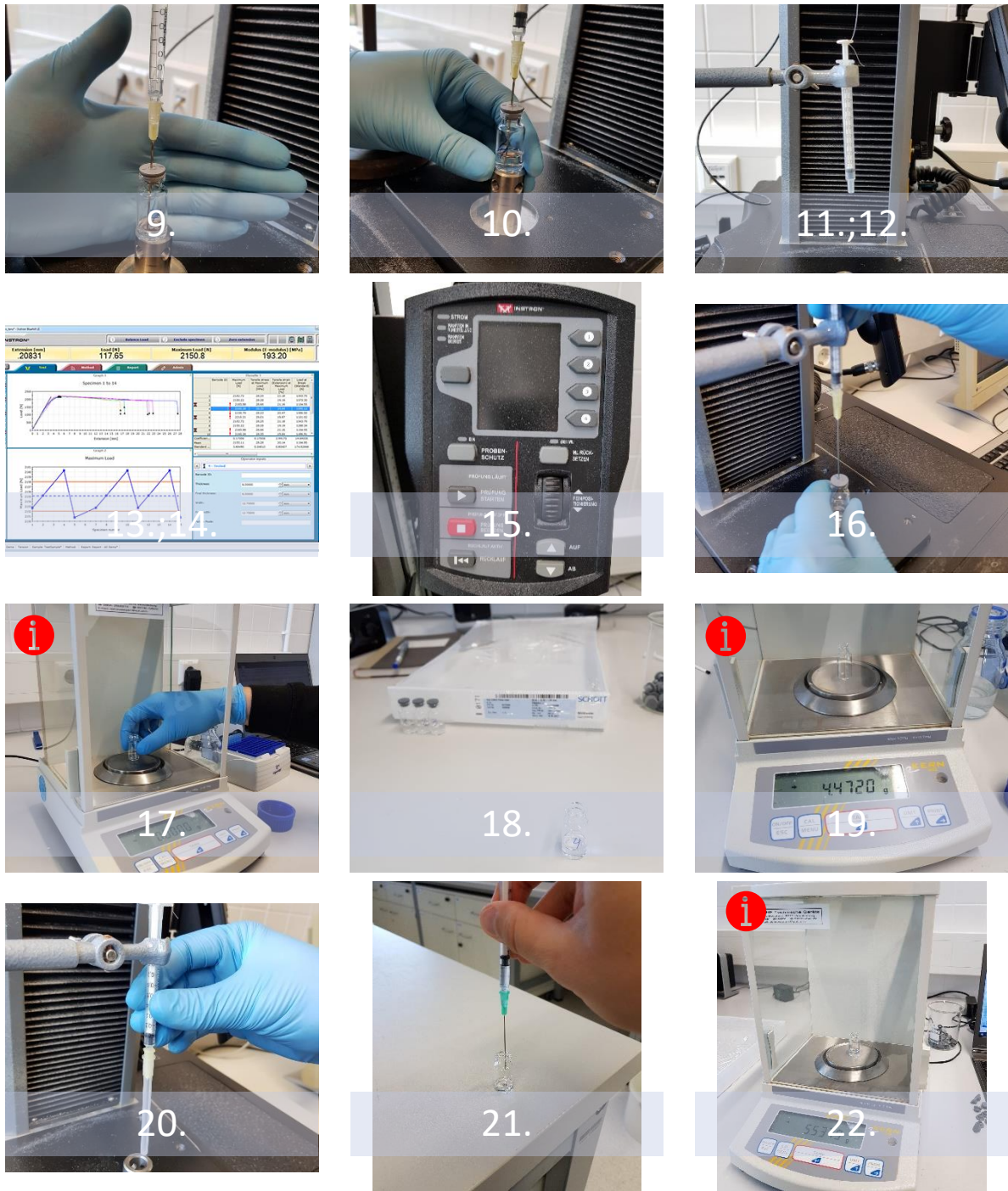
Figure 3-16: Procedure steps - Instron (steps with a red information sign are the ones in which data is collected); steps 1-8 in Figure 3-5
