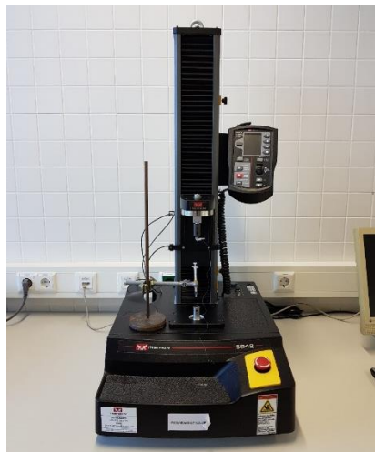
Figure 3-9: Instron™ 5942 Series® Single Column Table-top Testing System, used in this experiment
