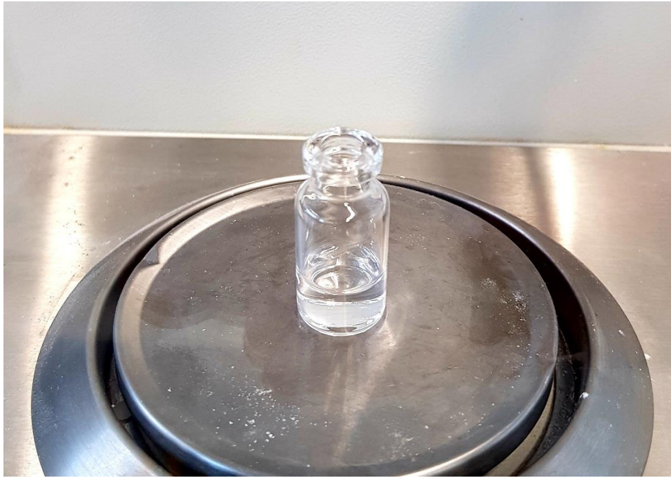
Figure 3-1: Schoot™ 2.00 mL Fiolax® clear, used in this experiment
