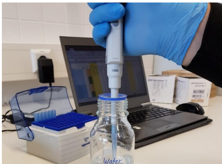
Figure 3-6: Eppendorf™ Research® plus Single-Channel; Blue; 100-1000 \mu\text{L} with Eppendorf™ epT.I.P.S.® 1 000 \mu\text{L} , used in this experiment
