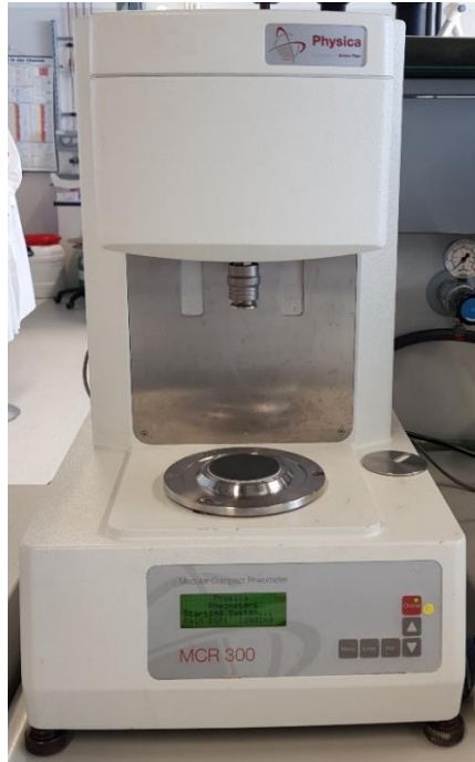
Figure 3-10: Anton Paar™ Physica® MCR 300 Rheometer with Anton Paar™ CP50-2® Measuring Cone, used in this experiment
