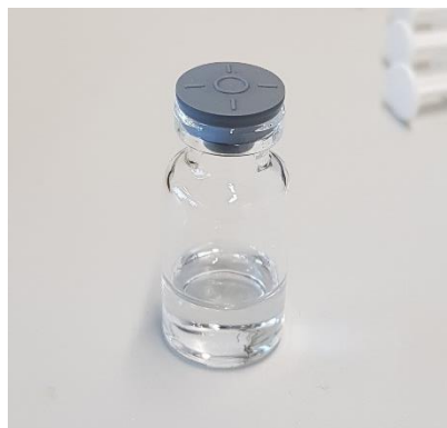
Figure 3-2: A vial with West™ Envision ® 13 mm stopper, used in this experiment
