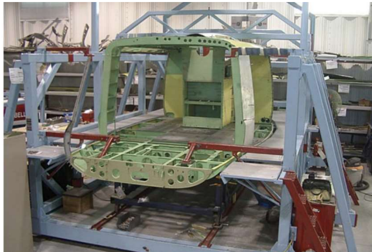
Figure 16: Example for a subassembly jig of the Bell 412, Source: Malaysian Institute of Aviation Technology (2014), p. 16.
