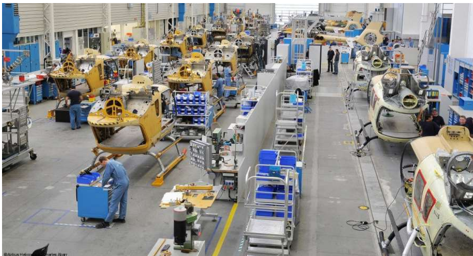
Figure 17: Example for a Final Assembly Line of the H135 in Germany, Source: Airbus S.A.S. (2015), online source [31.10.2018].
