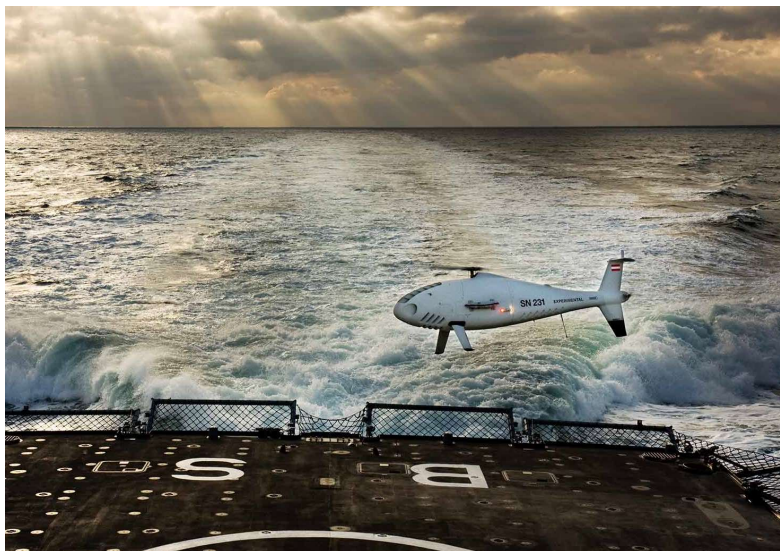
Figure 37: Schiebel's S-100 Camcopter on a maritime test flight, Source: Schiebel (2019), online source [28.1.2019].
