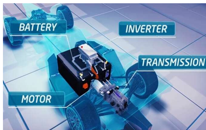
FIGURE 43: LONGITUDINAL ENGINE ON A FORMULA E CAR, ONLINE SOURCE: ABB FORMULA E (2016), [ACCESSED ON 20 NOVEMBER 2018]
