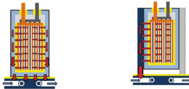
FIGURE 23: HEAT FLUX WITH BOTTOM COOLING (ON THE LEFT) AND WITH THE AID OF LATERAL FINS (ON THE RIGHT), SOURCE WIEBELT ET AL. (2009), P. 14
