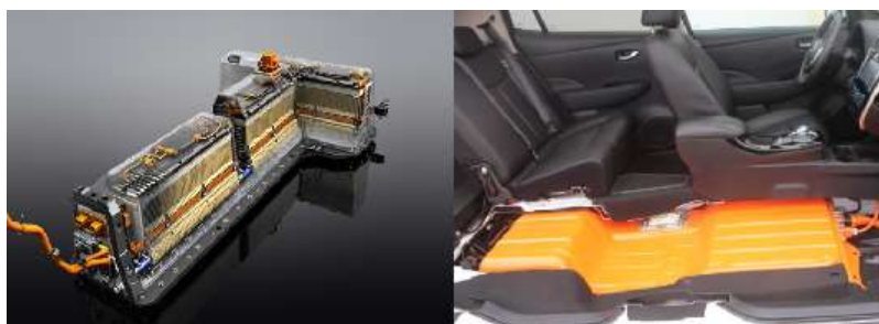
FIGURE 21: T-SHAPE OF THE BATTERY PACK IN THE CHEVROLET VOLT (2012) ON THE LEFT, MAT-SHAPE IN THE NISSAN LEAF (2013) ON THE RIGHT, ARCUS (2016), ONLINE SOURCE [ACCESSED ON 25 NOVEMBER 2018]
