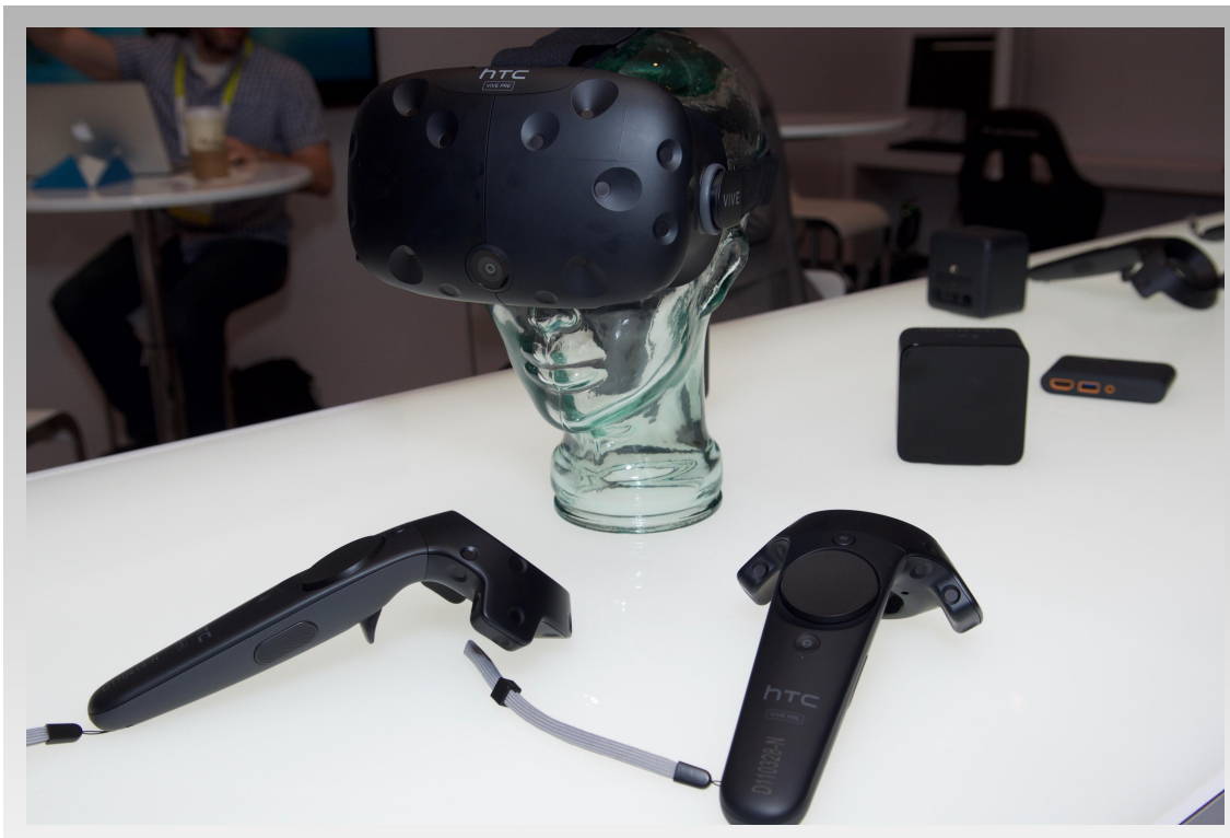
Figure 5.2: The HTC Vive consists of a Head Mounted Display (HMD), two handheld wireless controllers and two tracking stations. (source: https://commons.wikimedia.org/wiki/File:Vive_pre.jpeg )
