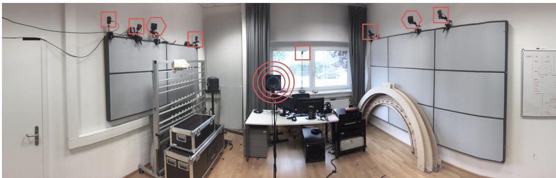
Figure 2.1 – The position of the real loudspeaker is the same as in the virtual studio and is marked with red circles. Red rectangles identify OptiTrack cameras, and red hexagons indicate the two HTC VIVE cameras.
