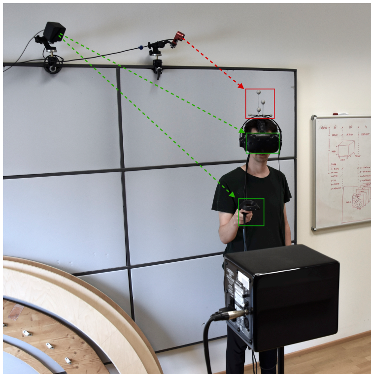
Figure 2.2 – The setup for the participants during the experiment. Red = Optitrack system; Green = HTC VIVE system. Both systems were used to gather position and orientation data. The OptiTrack system was used only when the participants did not wear the HMD. In front of the participant, one can see the real loudspeaker.
